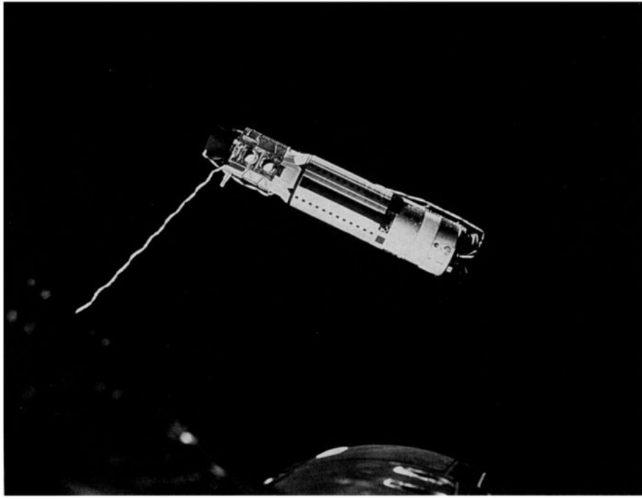
The view from Gemini 11's window of the Agena rocket with which the Gemini crew is practicing rendezvous and tethered station keeping.
