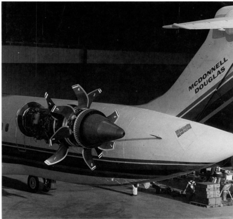
One version of the NASA-developed propfan, mounted on a production airliner for flight tests.
