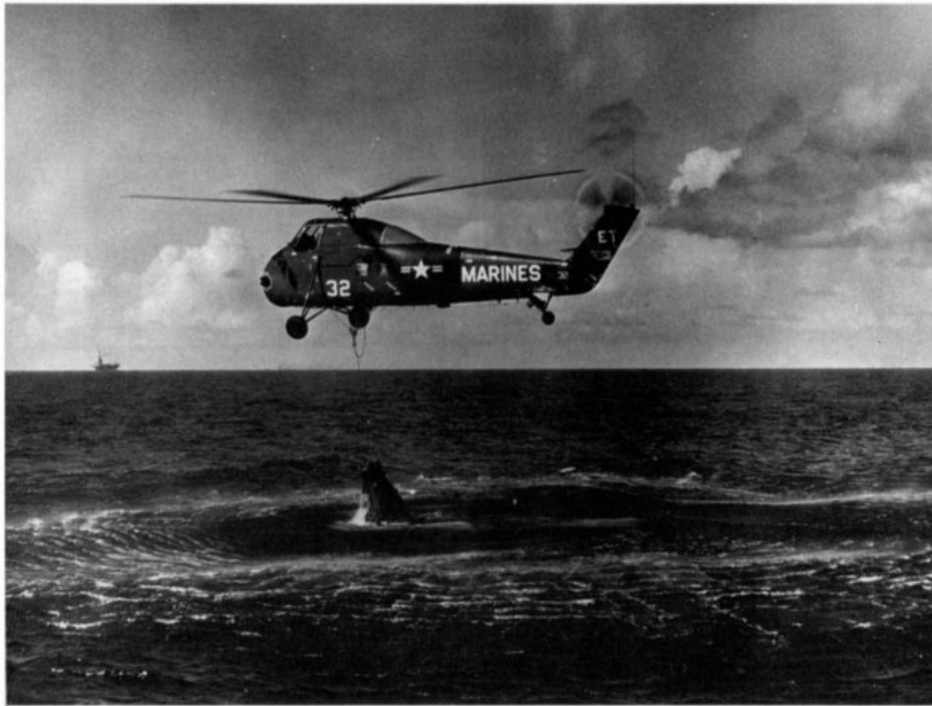
Mercury, Atlas, and Apollo crew capsules all splashed down into the Pacific, to be retrieved by helicopter. The Sikorsky UH-34D lost its struggle with Grissom's capsule, which sank after the astronaut scrambled out.
