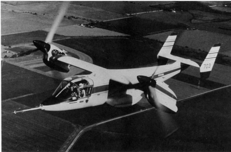
The XV-15 tilt rotor research aircraft. For takeoff (above), the crafts rotors are horizontal to provide lift, then they pivot forward (bottom) to a full verticle position to give cruising speeds twice those of conventional helicopters.
