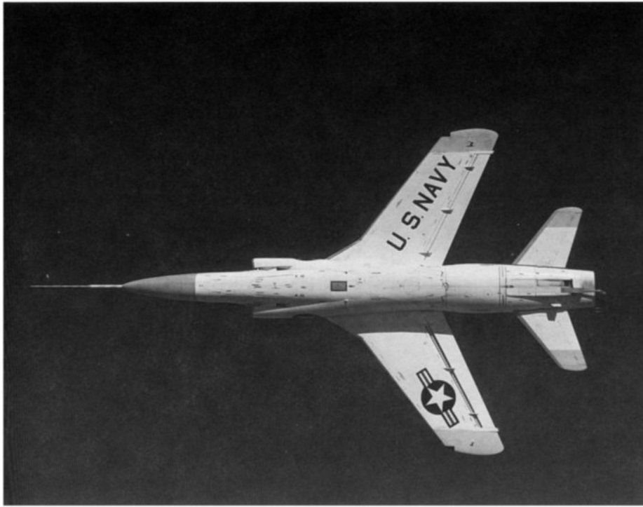
This photo taken from below the Grumman F-11 Navy fighter illustrates the way in which the area-ruled fuselage was adapted to production aircraft.
