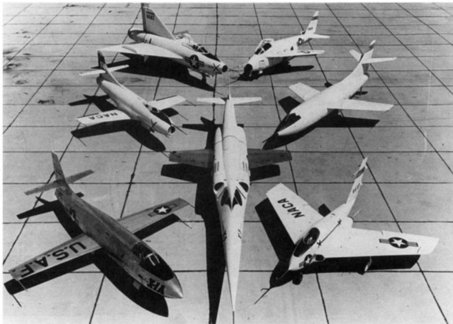
This Group portrait displays typical high-speed research aircraft that made headlines at Muroc Flight Center in the 1950s. The Bell X-1A (lower left) had much the same configuration as the earlier X-1. Joining the X-1A were (clockwise): the Douglas D-558-I Skystreak; Convair XF92-A, Bell X-5 with variable sweepback wings, Douglas D-558-II Skyrocket; Northrop X-4; and (center) the Douglas X-3
