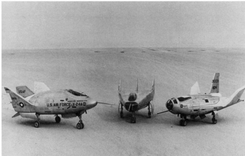
Three lifting body configurations grouped on the dry lake bed at Flight Research Center. Left to right: the X-24, M-2, and HL-10.
