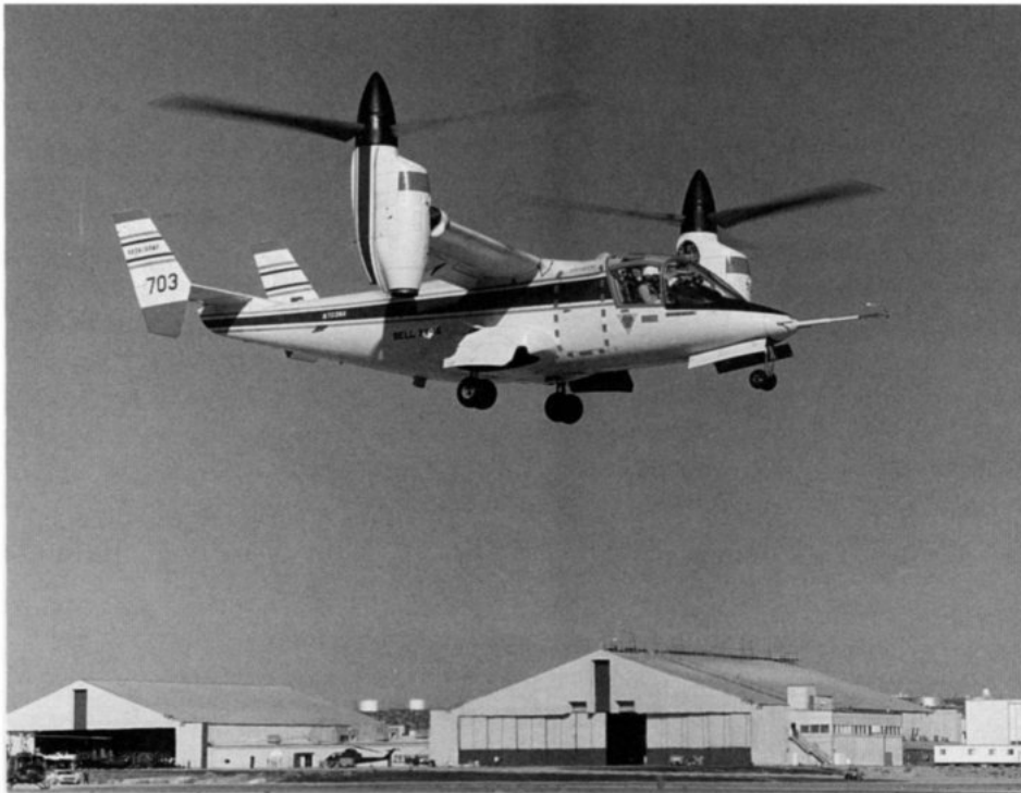
The XV-15 tilt rotor research aircraft. For takeoff (above), the crafts rotors are horizontal to provide lift, then they pivot forward (bottom) to a full verticle position to give cruising speeds twice those of conventional helicopters.
