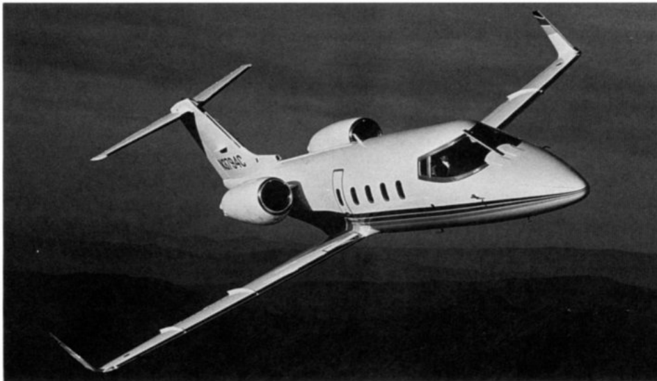
Winglets were incorporated into the design of the Learjet model 55 (photo courtesy of Gates Learjet Corporation).
