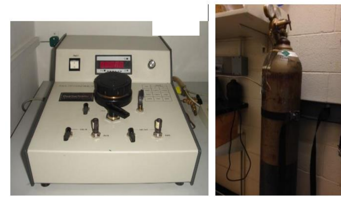
Figure. 3 Multi-pycnometer with nitrogen gas tank
