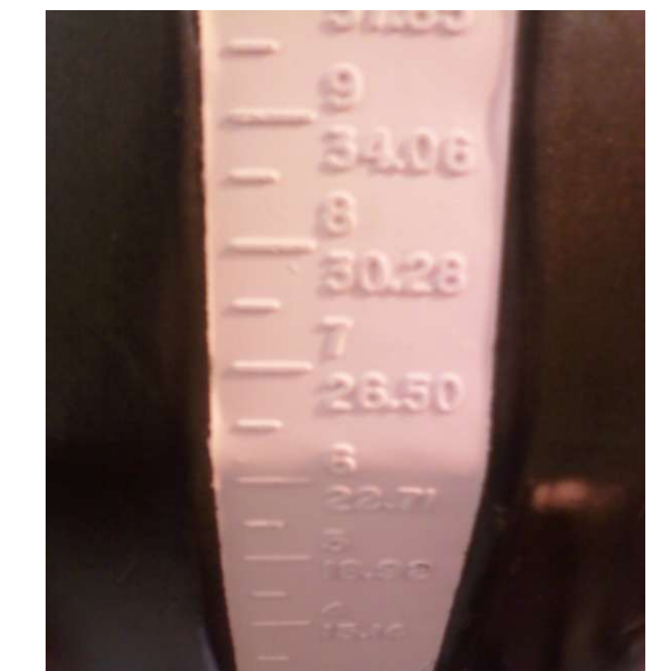
Figure 5 shows the scale on the side of the poly tank. It is scaled in gallons
