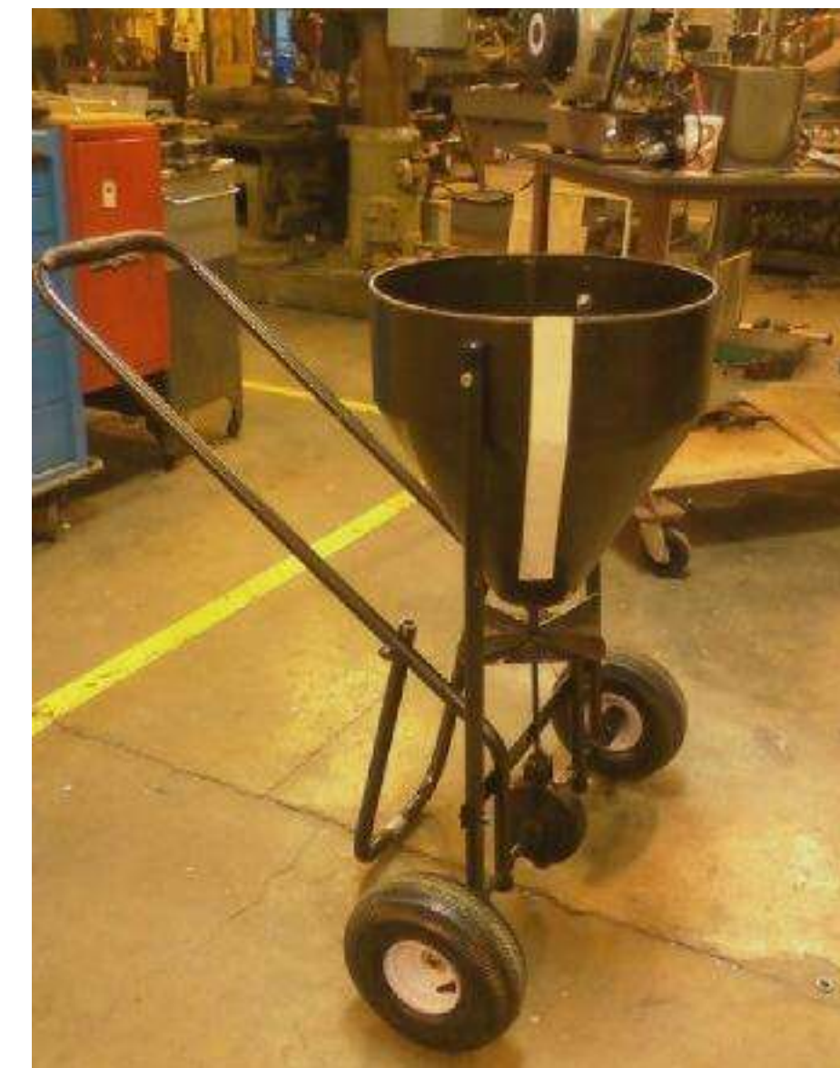
Figure 6 shows the completed spreader
