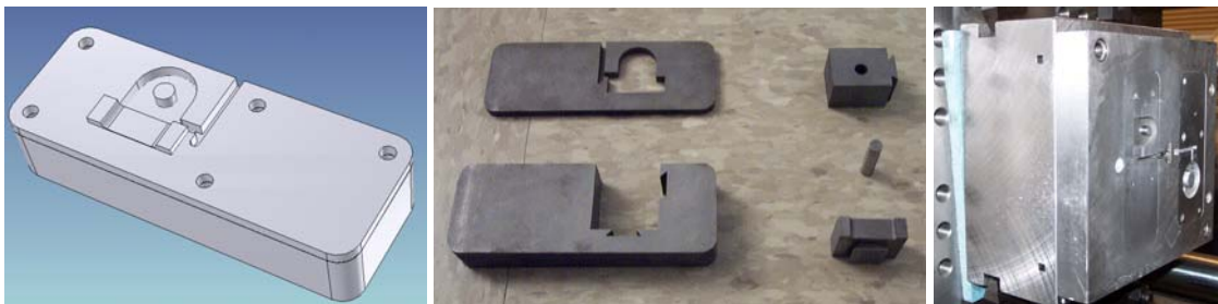
Figure 2: From right- 2a:CAD model of the mold, 2b:all pieces of this insert mold were made with wireEDM, 2c:insert mold mounted in the injection molding machine.
