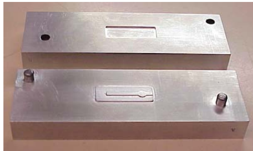
Figure 10: Micro mold for thermo-forming process made with wirePATH method.
