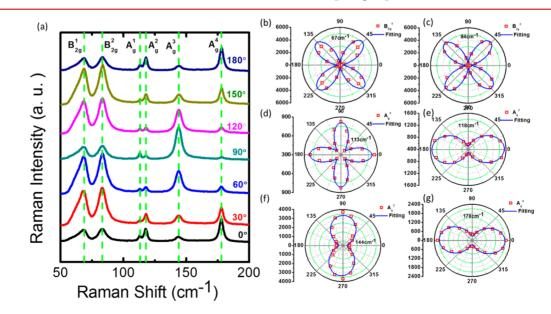
**Figure 2.** (a) Raman spectra of a fresh exfoliated flake evolving with rotating angle between the flake and incident polarization. (b-g) are corresponding to  $B_{2g}^1$ ,  $B_{2g}^2$ ,  $A_g^1$ ,  $A_g^2$ ,  $A_g^3$ , and  $A_g^4$  Raman modes which are located at 67, 84, 113, 118, 144, and 178 cm<sup>-1</sup>. The fitted curves are described as eq 3 and 4.
