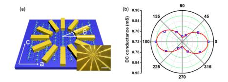
**Figure 3.** Angle-resolved DC conductance measurements on  $ZrTe_5$  flake. (a) Schematic view of device structure. Inset: optical image of a real device. Scale bar is 10  $\mu$ m. (b) Angle-dependent DC conductance. The data points are fitted with the equation:  $\sigma_{\theta} = \sigma_x \sin^2 \theta + \sigma_y \cos^2 \theta$ .
