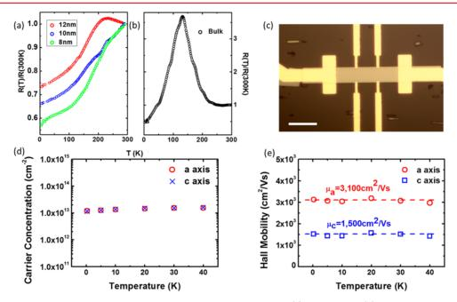
**Figure 4.** Low-temperature transport measurements. Resistivity vs temperature curve on (a) few-layer and (b) bulk  $ZrTe_5$  samples. The resistivity is normalized based on room temperature values. (c) Optical image of the Hall-bar device. The scale bar is 10  $\mu$ m. Temperature dependence of (d) carrier concentration and (e) Hall mobility along two principal axis.
