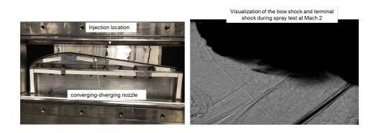
Research is underway at a more fundamental level at Mach 2 to characterize sprays in a fully optical accessible test section. The liquid jet is monitored using multiple techniques such as kHz shadowgraphy, backlit imaging, and Mie Scattering. This figure shows some experiments performed in the Linear Experimental Aerothermal Facility (LEAF).
