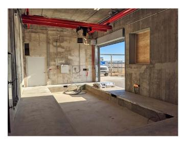
lab including tall ceilings with overhead cranes for ease of assembly, bedplates flush-mounted to the floors, and an overhead fan to prevent hot air from accumulating in the test cells. With research equipment being delivered in the next couple of months, the team expects to accomplish the first spin of the rig this year.
