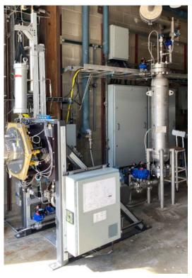
existing rocket cell data acquisition system to read further high frequency and low frequency data channels. The stand also makes use of Coriolis flow measuring devices which provide density and flow rates in real time. Hotfires conducted on Stand A have already provided the test sponsor with data that has resulted in marked improvement of the sponsor's development articles.
