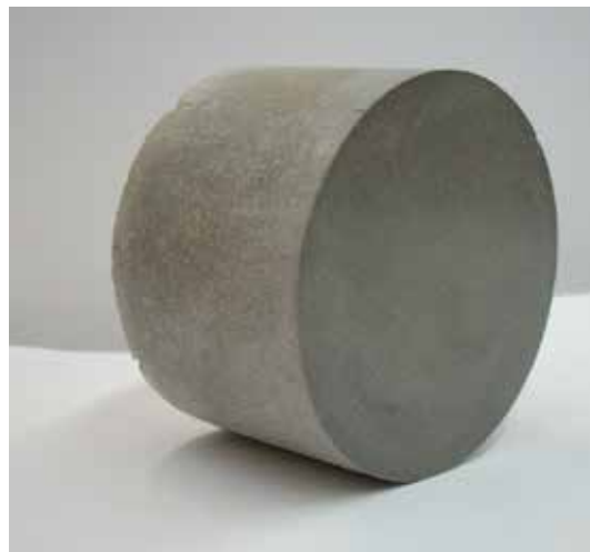
Figure 1. Photograph of a 5-cm-diameter CNC-cement sample produced for the study, from which small test specimens were cut for analytical and mechanical testing.
