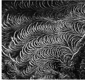
Diffused subcritical matrix cracks (white)
