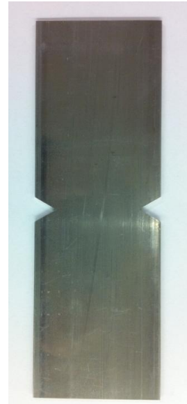
Figure 2. Notched steel plate
