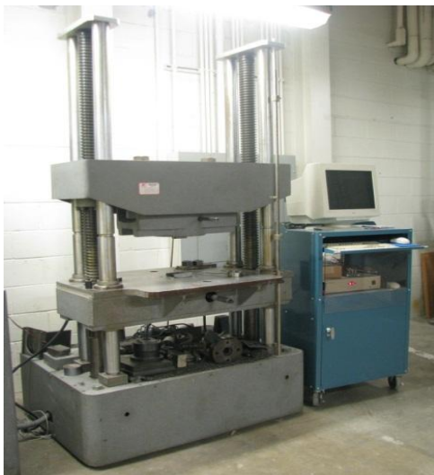
Figure 3. Servo-hydraulic machine for tension test
