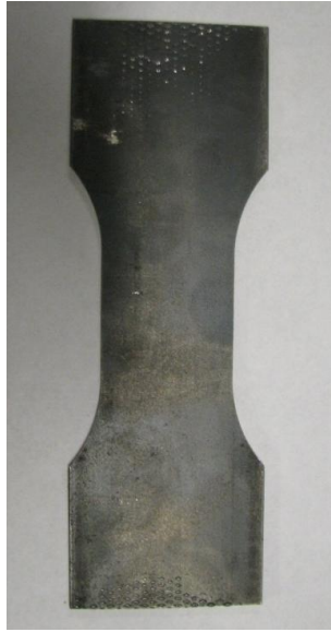
Figure 1. Un-notched steel plate
