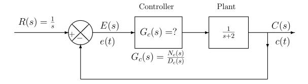
Figure 2: A closed-loop control system of Example 1.
