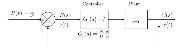
Figure 3: A closed-loop control system of Example 2.
