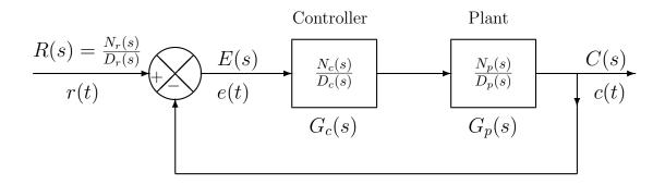
Figure 1: Block diagram of a closed-loop control system.
