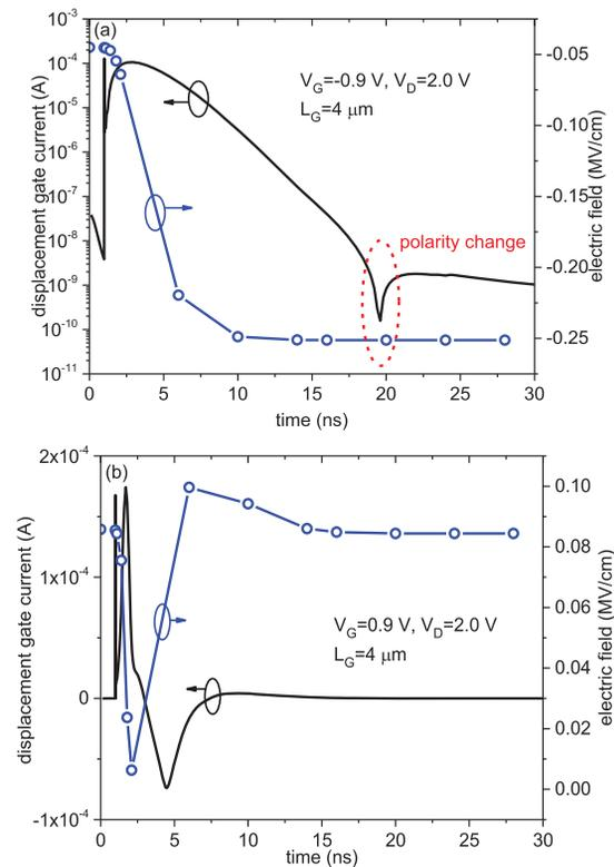
Fig. 5. Displacement gate current and electric field in  $\text{La}_2\text{O}_3$  as a function of time at (a)  $V_G = -0.9$  V; (b)  $V_G = 0.9$  V.
