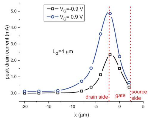
Fig. 15. Simulated peak drain current along a horizontal cut line at two different gate biases.
