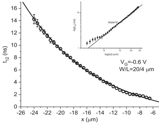
Fig. 11. The time difference between the first peak and second peak of the drain transients versus the strike location. Here the center of the gate is taken as the origin and the drain is in the negative  $x$  direction. The error bar represents one standard deviation of the transients taken at a single location. The inset plots the same data on a log-log scale.
