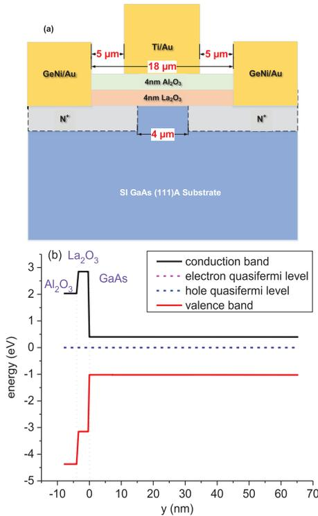
Fig. 1. (a) Schematic cross section of the device with  $L_G = 4 \mu\text{m}$ ; (b) band diagram along a vertical cutline through the device oxide at  $V_G = V_D = V_S = 0 \text{ V}$ . The band diagram is generated from Sentaurus TCAD simulation.
