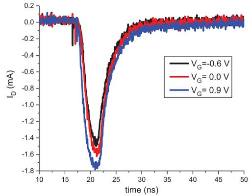
Fig. 13. Drain transients at different gate biases at a location of  $x = -9$   $\mu\text{m}$ .  $V_{TH} = 0.3$  V,  $V_D = 2.0$  V. The inset shows the tail portion of the transient.
