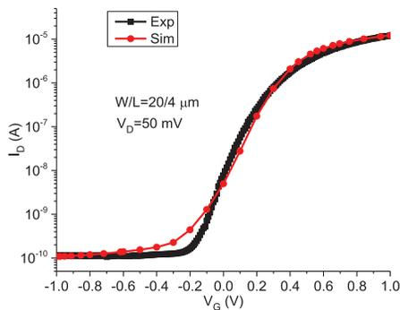
Fig. 2. Measured and simulated  $I_D - V_G$  transfer characteristics.  $V_D = 50 \text{ mV}$  during measurement. Simulation is done with Sentaurus TCAD tools.
