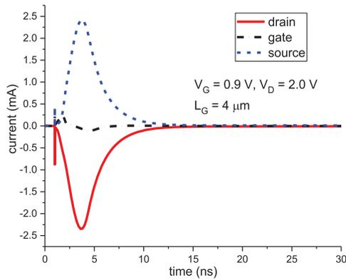
Fig. 6. Simulated current transients at  $V_G = 0.9$  V,  $V_D = 2.0$  V when striking at  $x = -6$   $\mu\text{m}$ . The current is scaled by the width of 33  $\mu\text{m}$ .
