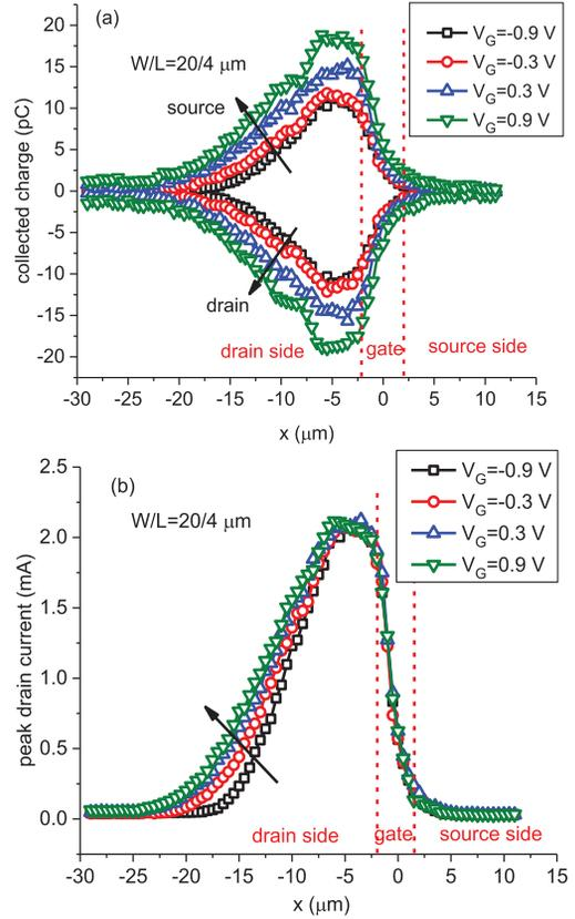
Fig. 12. (a) Collected charge, and (b) peak drain current along a line scan at different gate biases.  $V_{TH} = 0.3$  V,  $V_D = 2.0$  V. In (a), the positive collected charge corresponds to the source, and the negative collected charge corresponds to the drain. The arrows show the trends vs. gate bias.
