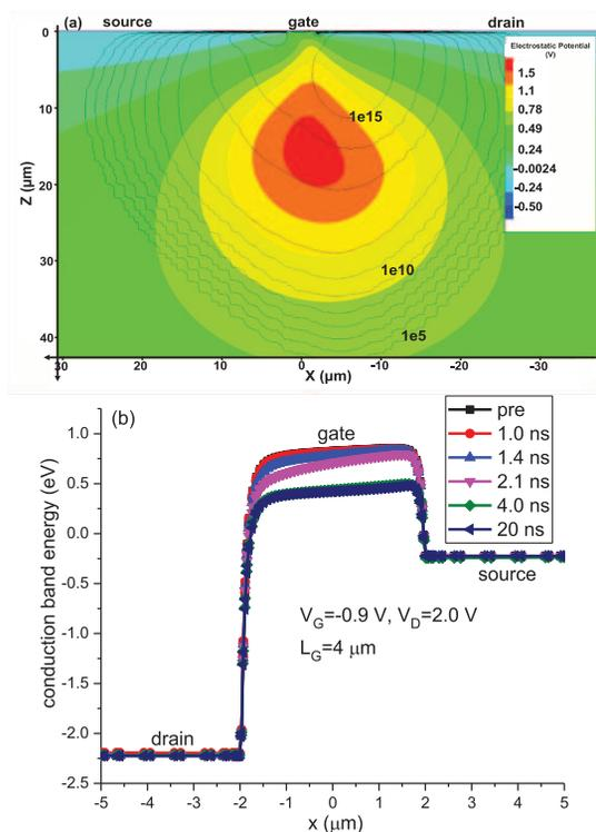
Fig. 8. (a) The color map shows the electrostatic potential difference and the contour plot shows the hole density difference between post-strike (4.0 ns) and pre-strike at  $V_G = -0.9$  V. (b) The conduction band energy is plotted along a horizontal outline at  $z = 50$  nm at different times.
