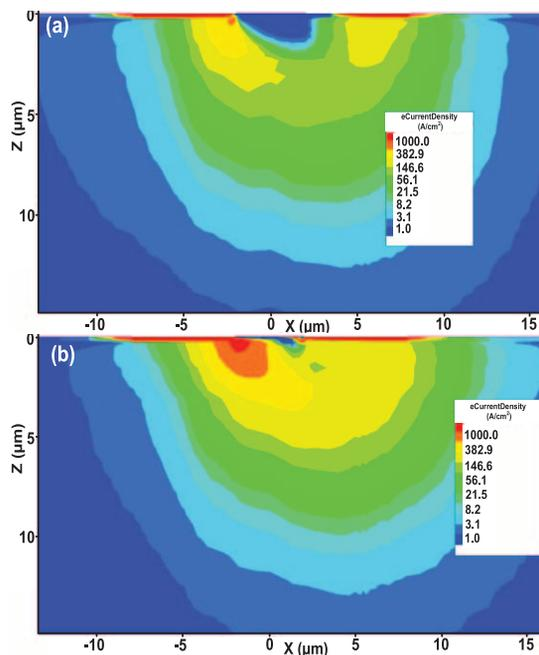
Fig. 14. Electron current density difference between post-strike (4.0 ns) and pre-strike at (a)  $V_G = -0.9$  V; (b)  $V_G = 0.9$  V.
