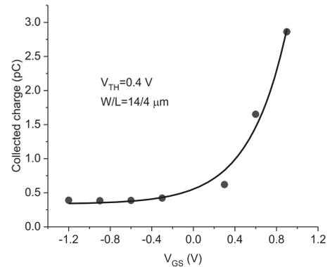
Fig. 7. Drain collected charge as a function of gate bias under oxygen ion irradiation.  $V_D = 2$  V during irradiation.
