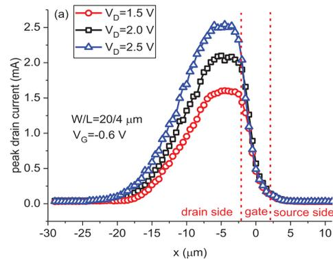
Fig. 16. Peak drain current along a line scan vs. drain biases.  $V_{TH} = 0.3$  V.
