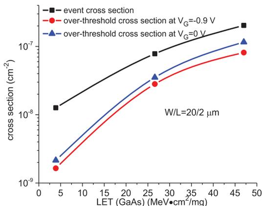
Fig. 9. The event cross section and the over threshold cross section at  $V_G = -0.9$  V and  $V_G = 0$  V as a function of LET.  $V_D = 2$  V during irradiation.
