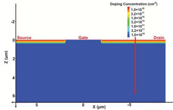
Fig. 3. Device model used in 2D TCAD simulation. Here the drain is in the negative  $x$  direction and source is in the positive  $x$  direction. The red arrow indicates the strike location,  $x = -6 \mu\text{m}$ . For the simulation, Sentaurus TCAD tools are used.
