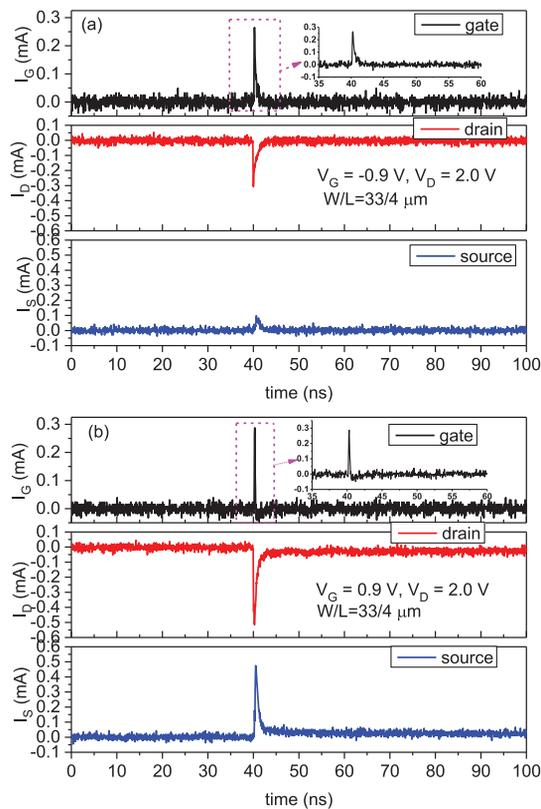
Fig. 4. Representative transients under oxygen ion irradiation at (a) OFF,  $V_G = -0.9$  V; (b) ON bias conditions;  $V_G = 0.9$  V for a device with  $L_G = 4$   $\mu\text{m}$ . For this device,  $V_{TH} = 0.4$  V. The inset of the figure shows the zoom into the magenta box region.
