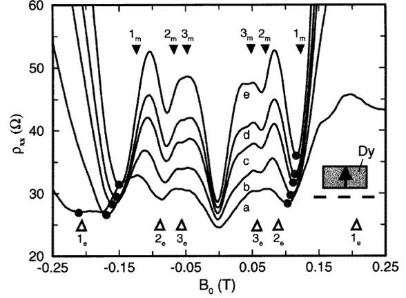
**Figure 3.** Low-field  $\rho_{xx}$  traces for a Dy grating with  $a = 1 \mu\text{m}$  taken at 4.2 K for  $M \parallel \hat{z}$  (see inset) showing the shift of the  $\rho_{xx}$  minima with increasing  $B^{\max}$ . Full triangles mark the position of the *magnetic* flat-band condition (subscript ‘m’) while the open triangles mark the *electric* ones (subscript ‘e’). The full circles highlight the positions of the  $\rho_{xx}$  minima.
