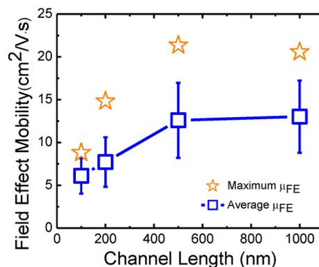
**Figure 7.** Average and maximum values of intrinsic carrier mobility at all channel lengths. The impact of contact resistance is subtracted from the data. The maximum values are 8.8, 14.8, 21.4, and 20.6  $\text{cm}^2/\text{V}\cdot\text{s}$  for 100 nm, 200 nm, 500 nm, and 1  $\mu\text{m}$  channel length devices.
