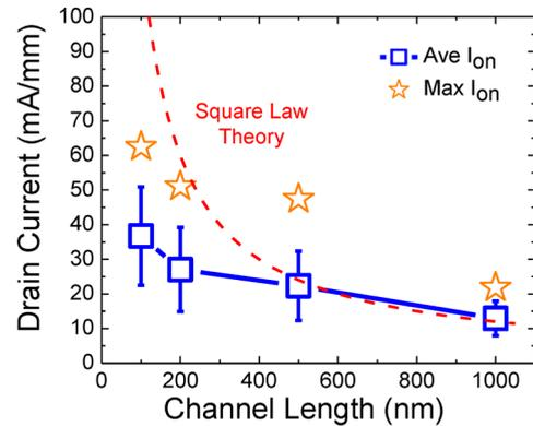
**Figure 4.** Averaged values of maximum drain current at all channel lengths. Maximum values in measurement are also plotted. Red dashed line shows Square Law Model prediction of channel length-dependent drain current that fits long channel device performance. The deviation at short channel regions is due to contact resistance and velocity saturation.
