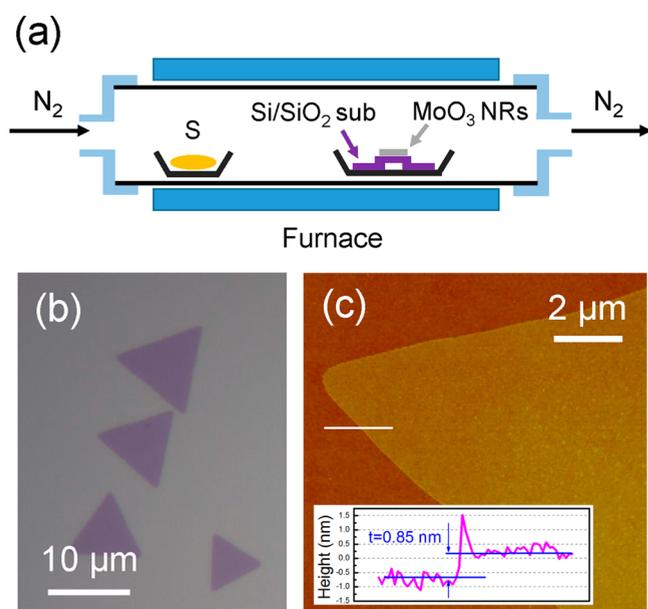
**Figure 1.** (a) Schematic view of CVD synthesis of monolayer MoS<sub>2</sub> in a furnace. (b) Optical micrograph of single crystalline monolayer CVD MoS<sub>2</sub>. Scale bar is 10 μm. (c) AFM image of a synthesized MoS<sub>2</sub> crystal showing good single layer thickness uniformity. Scale bar is 2 μm.
