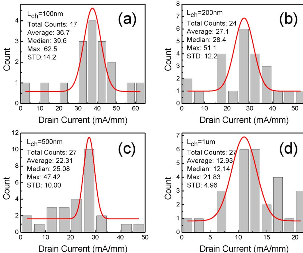
**Figure 3.** Maximum drain current distributions of (a) 100 nm, (b) 200 nm, (c) 500 nm, and (d) 1  $\mu$ m devices extracted from back-gate modulation. Average values of  $36.7 \pm 14.2$ ,  $27.1 \pm 12.2$ ,  $22.3 \pm 10.0$ , and  $12.9 \pm 5.0$  mA/mm for 100 nm, 200 nm, 500 nm, and 1  $\mu$ m channel lengths are acquired, respectively.
