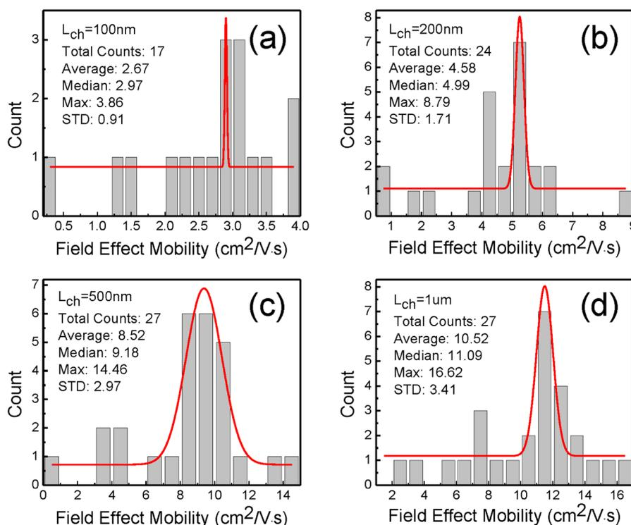
**Figure 6.** Extrinsic field-effect mobility distributions of (a) 100 nm, (b) 200 nm, (c) 500 nm, and (d) 1  $\mu\text{m}$  devices from back-gate modulation. Carrier mobilities are extracted from transconductance at low drain bias ( $V_{ds} = 0.05$  V). Average values of  $2.67 \pm 0.91$ ,  $4.58 \pm 1.71$ ,  $8.52 \pm 2.97$ , and  $10.52 \pm 3.41$   $\text{cm}^2/\text{V}\cdot\text{s}$  for 100 nm, 200 nm, 500 nm, and 1  $\mu\text{m}$  channel length are calculated.
