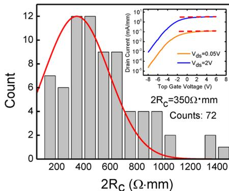
**Figure 5.** Intrinsic contact resistance distributions in all top-gated devices. An expectation of 350  $\Omega\cdot\text{mm}$  is predicted by normal distribution. Inset: Typical transfer curves from a top-gated device showing early current saturation.
