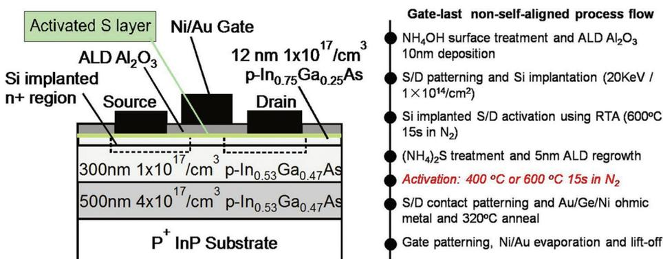
FIG. 1. (Color online) Schematic cross section and fabrication process of a non-self-aligned inversion-mode n-channel  $\text{In}_{0.75}\text{Ga}_{0.25}\text{As}$  MOSFET with gate-last process. 400 or 600 °C PDA process after gate dielectric regrowth is added to investigate the thermal stability of the  $(\text{NH}_4)_2\text{S}$  treatment.
