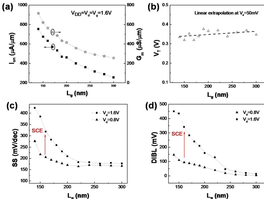
FIG. 8. (Color online) (a) on-current and peak transconductance at  $V_{DD} = 1.6$  V (b) linear extrapolated ( $V_d = 50$  mV) threshold voltage (c) subthreshold swing (SS) and (d) drain-induced barrier (DIBL) scaling metrics for gate-first self-aligned  $\text{In}_{0.65}\text{Ga}_{0.35}\text{As}$  MOSFET with Ni/Au metal gate.
