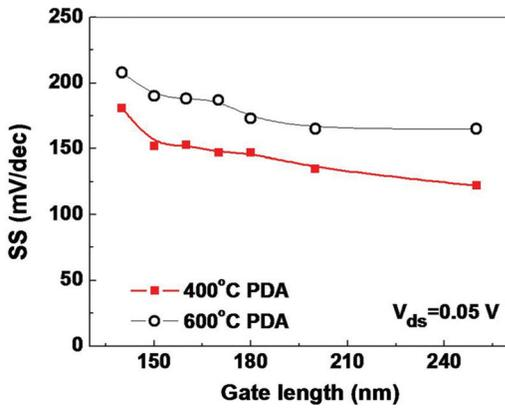
FIG. 5. (Color online) Subthreshold swing of a gate-last  $\text{In}_{0.75}\text{Ga}_{0.25}\text{As}$  MOSFETs with 400 or 600°C PDA after gate oxide deposition, showing a  $\sim 20\%$  degradation at 600°C PDA condition.
