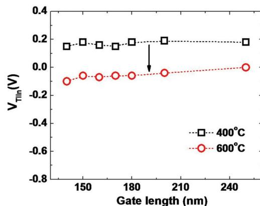
FIG. 4. (Color online) Linear extrapolated ( $V_{ds} = 50$  mV) threshold voltage for a gate-last  $\text{In}_{0.75}\text{Ga}_{0.25}\text{As}$  MOSFET with various gate lengths. A consistent  $-0.3$  V  $V_T$  shift is observed for all devices after 600 °C PDA.
