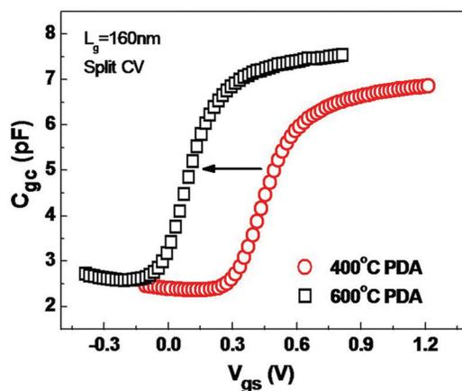
FIG. 3. (Color online) Split CV measurement of an  $L_g = 160$  nm gate-last  $\text{In}_{0.75}\text{Ga}_{0.25}\text{As}$  MOSFET. The inversion threshold shifts  $\sim 0.3$  V to a negative gate voltage for 600 °C PDA condition, with a  $\sim 10\%$  increase in  $C_{gc}$ .
