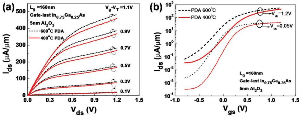
FIG. 2. (Color online) (a) output and (b) transfer characteristics of an  $L_g = 160$  nm gate-last  $\text{In}_{0.75}\text{Ga}_{0.25}\text{As}$  MOSFET with 400 or 600 °C PDA process after gate dielectric deposition.
