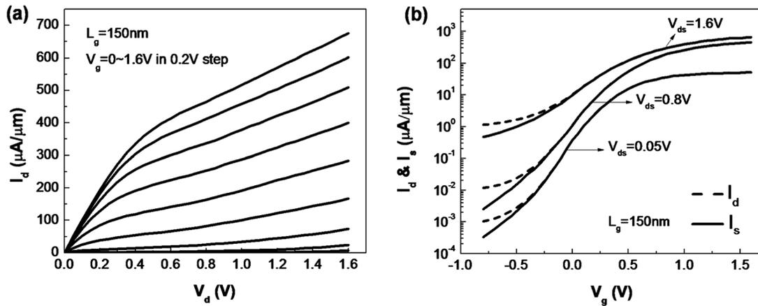
FIG. 7. (a) output and (b) subthreshold characteristics of an  $L_g = 150$  nm gate-first self-aligned  $\text{In}_{0.65}\text{Ga}_{0.35}\text{As}$  MOSFET with Ni/Au metal gate.
