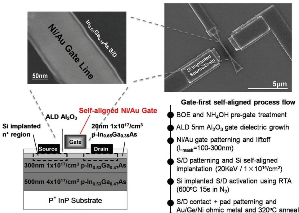
FIG. 6. (Color online) Schematic cross section and fabrication process of a self-aligned inversion-mode n-channel  $\text{In}_{0.65}\text{Ga}_{0.35}\text{As}$  MOSFET with a gate-first process. Insets show the SEM images of Ni/Au gate line and top-view device structure of a typical  $L_g = 150 \text{ nm}$  device.
