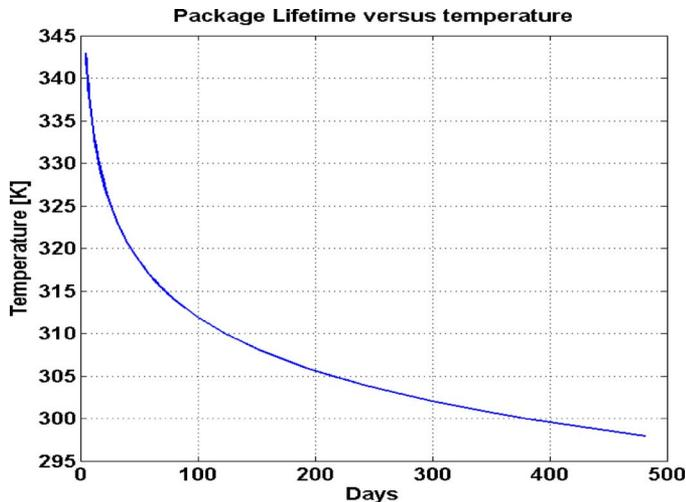
Fig. 13. Package lifetime versus testing temperature.
