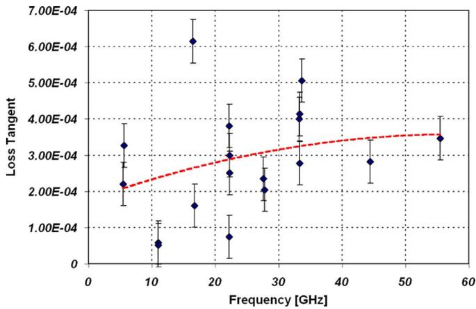
Fig. 6. Loss tangent of Parylene-N extracted from measurements.
