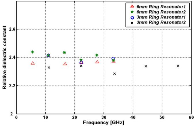
Fig. 5. Relative dielectric constant of Parylene-N extracted from measurements.
