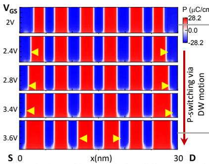
**Fig. 14:**  $P$  profile in FE for different  $V_{GS}$  in FEFET showing DW motion-based P-switching. Yellow arrow points towards the DW motion
