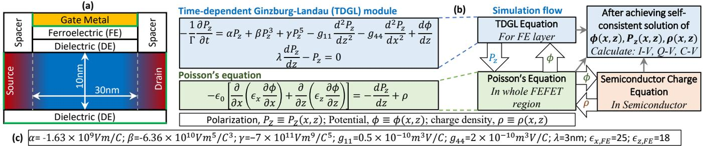
Fig. 3: (a) Simulated FeFET structure, (b) self-consistent simulation flow among TDGL, Poisson's and semiconductor (silicon) charge equations (c) FE parameters used in FEFET simulation. For the simulation of metal-FE-insulator-metal (MFIM) stack only Poisson's and TDGL equations are used.
