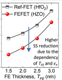
**Fig. 25:** Subthreshold swing (SS) for different  $T_{FE}=T_{\text{HfO}_2}$  showing more SS reduction in FEFET.
