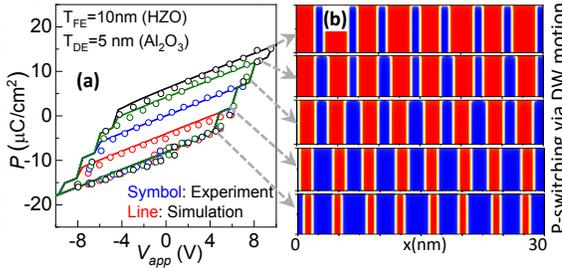
Fig. 6: (a) Partial  $P$ -switching characteristics in MFIM stack. (b) Corresponding  $P$  profile signifying domain nucleation and domain-wall (DW) motion based  $P$ -switching.  $T_{FE} = 10 \text{nm}$ ,  $T_{DE} = 3 \text{nm}$ .
