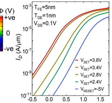
**Fig. 16:** (a)  $I_D-V_{GS}$  characteristics of FEFET with  $T_{FE}=5\text{nm}$  showing multi-level memory operation.
