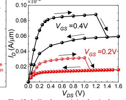
**Fig. 18:**  $I_D-V_{DS}$  characteristics showing hysteretic behavior. The  $P$  profile of the FE layer is shown for  $V_{DS}=0.6\text{V}$  considering (b) forward sweep and (c) reverse  $V_{DS}$  sweep. Due to the P-switching near drain side the drain barrier height increases leading to a lower current in reverse sweep compared to forward sweep.
