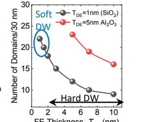
Fig. 8: Number of domains as a function of  $T_{FE}$  for different  $T_{DE}$  showing that the domain pattern becomes denser with decreasing  $T_{FE}$ .
