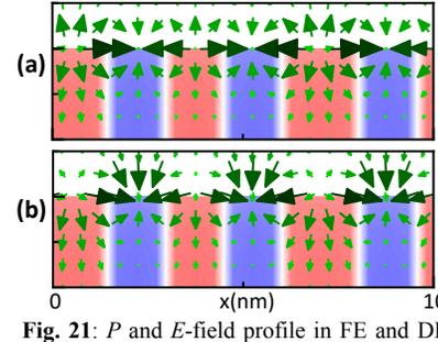
**Fig. 21:**  $P$  and  $E$ -field profile in FE and DE layer of the MFIS stack at (a)  $0\text{V}$  and (b)  $-0.5\text{V}$  showing the transformation of stray in-plane  $E$ -field to out-of-plane  $E$ -field due to the magnitude change of  $P$ . This phenomena leads to extra charge in FE-DE interface leading to enhanced effective  $\epsilon_r$  in FE layer.
