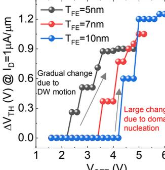
**Fig. 17:** (a) Memory window ( $\Delta V_{TH}$ ) for different  $T_{FE}$  and  $V_{SET}$  showing that MW increases with the increase in  $T_{FE}$ .
