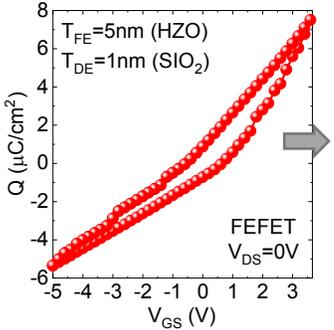
**Fig. 13:** Simulated  $Q-V_{GS}$  of FEFET showing hysteretic characteristics for  $T_{FE}=5\text{nm}$  due to DW motion.
