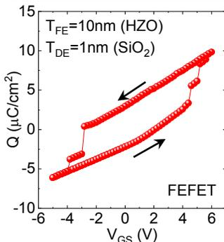
Fig. 9: Simulated gate charge ( $Q$ ) vs  $V_{GS}$  at  $V_{DS} = 0 \text{V}$  of FEFET showing hysteretic characteristics demonstrating the  $P$ -switching in the FE layer.
