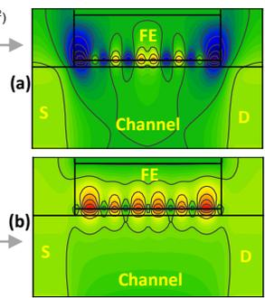
**Fig. 15:** FEFET Potential profile at  $V_{GS}=0\text{V}$  after (a)  $V_{RESET}=-3.6\text{V}$  and (b)  $V_{SET}=3.6\text{V}$  showing P-switching induced change in channel potential.
