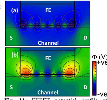
Fig. 11: FEFET potential profile at  $V_{GS} = 0 \text{V}$  after (a)  $V_{RESET} = V_{GS} = -5 \text{V}$  and (b)  $V_{SET} = V_{GS} = 6 \text{V}$  showing  $P$ -switching induced change in channel potential as well as non-uniform potential in channel.
