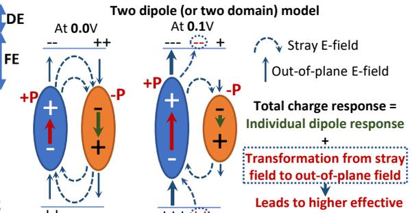
**Fig. 22:** Two dipole (or domain) scenario describing the origin of enhanced- $\epsilon_r$  of hard multi-domain thin FE film as a voltage induced change in dipole interaction associated electric field.
