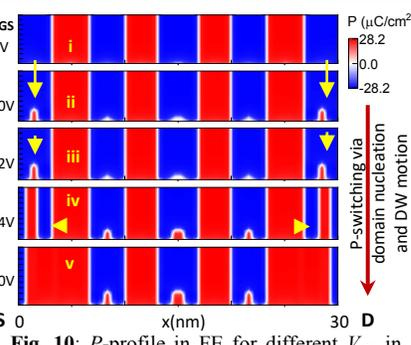
Fig. 10:  $P$ -profile in FE for different  $V_{GS}$  in FEFET showing domain nucleation (i-iv) followed by DW motion (iv-v) based  $P$ -switching. Note:  $P$ -switching is dominant near the source (S) and drain (D) region.
