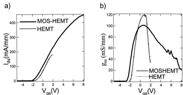
FIG. 4. Measured (a) transfer and (b) transconductance characteristics measured with the MOS-HEMT (solid line) and HEMT (dashed line) in saturation ( $V_{ds}=10$  V).
