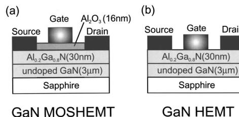
FIG. 1. Cross sections of (a) an ALD  $\text{Al}_2\text{O}_3/\text{AlGaIn}/\text{GaN}$  MOS-HEMT and (b) a conventional  $\text{AlGaIn}/\text{GaN}$  HEMT of similar design.
