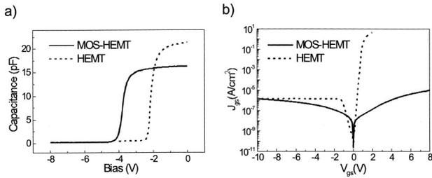
FIG. 2. Measured (a)  $C$ - $V$  characteristics and (b) gate leakage of the MOS-HEMT (solid line) and the baseline HEMT (dashed line).
