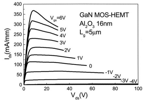
FIG. 3. Measured  $I$ - $V$  characteristics of the MOS-HEMT. The negative output conductance under high gate biases ( $V_{gs} \geq 0$ ) is due to self-heating.
