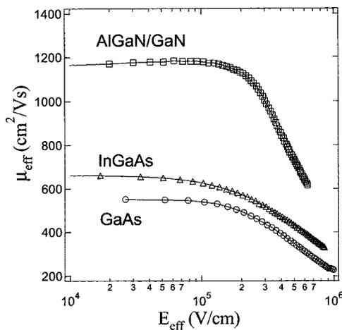
FIG. 5. Calculated effective 2D electron mobility vs. effective electric field at the AlGaIn/GaN (squares), Al<sub>2</sub>O<sub>3</sub>/InGaAs (triangles), and Al<sub>2</sub>O<sub>3</sub>/GaAs (circles) interfaces.
