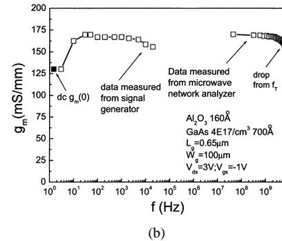
Fig. 3. (a) Drain current versus gate bias in both forward (dashed black line) and reverse (solid gray line) sweep directions. Dotted line is transconductance versus gate bias at  $V_{ds} = 3$  V. (b) Peak transconductance  $g_m$  versus frequency from dc to several gigahertz. The  $g_m$  is essentially constant for frequencies above 20 Hz, indicating that efficient charge modulation of the channel can be achieved over the entire useful frequency range of the device.
