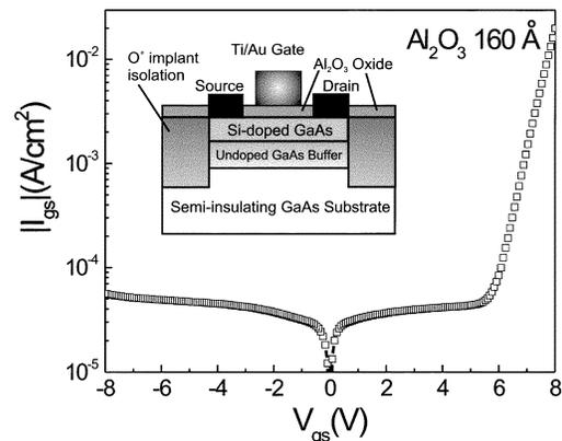
Fig. 1. Two-terminal gate  $I$ - $V$  characteristics of an  $\text{Al}_2\text{O}_3/\text{GaAs}$  MOSFET. Source and drain are grounded together. Inset: Schematic view of a depletion-mode n-channel GaAs MOSFET with ALD-grown  $\text{Al}_2\text{O}_3$  as gate dielectric.
