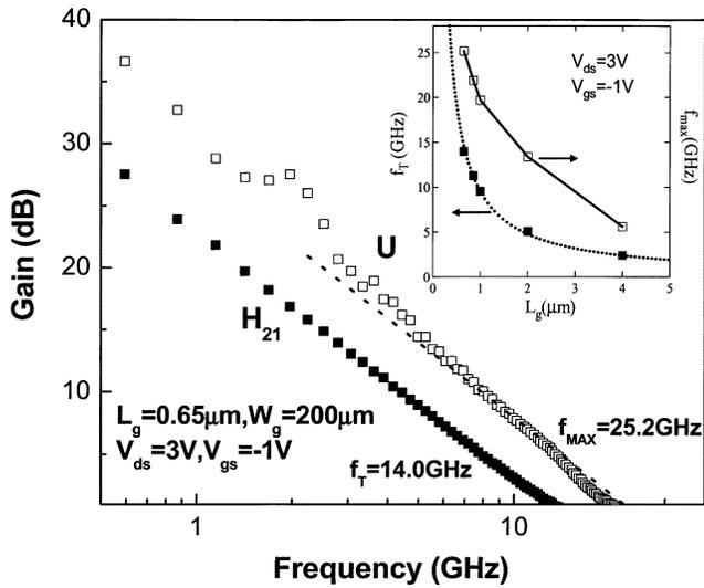
Fig. 4. RF characteristics of  $\text{Al}_2\text{O}_3/\text{GaAs}$  MOSFETs with gate length and width of 0.65 and 100  $\mu\text{m}$ , respectively. RF tester includes two identical devices with total gate length of 200  $\mu\text{m}$ . Inset:  $f_T$  and  $f_{MAX}$  for different gate lengths. The dashed line illustrates  $f_T = v_{sat}/2\pi L_g$ .
