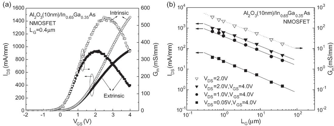
Fig. 2. (a) Extrinsic and intrinsic drain current and transconductance versus gate bias at  $V_{DS} = 2.0\text{ V}$ . (b) Extrinsic drain current at  $V_{GS} = 4.0\text{ V}$  and  $V_{DS} = 2.0\text{ V}$ ,  $V_{DS} = 1.0\text{ V}$ , or  $V_{DS} = 0.05\text{ V}$  versus  $L_G$  and the extrinsic peak  $G_m$  at  $V_{DS} = 2.0\text{ V}$  versus  $L_G$ . The solid and dotted lines are guided by eyes.
