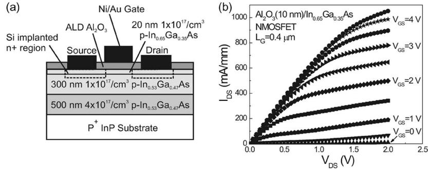
Fig. 1. (a) Cross section of an inversion-type E-mode  $\text{Al}_2\text{O}_3/\text{In}_{0.65}\text{Ga}_{0.35}\text{As}$  MOSFET. (b)  $I$ - $V$  characteristic of a  $0.4\text{-}\mu\text{m}$  gate-length  $\text{In}_{0.65}\text{Ga}_{0.35}\text{As}$  MOSFET with a  $10\text{-nm}$  ALD  $\text{Al}_2\text{O}_3$  as gate dielectric.
