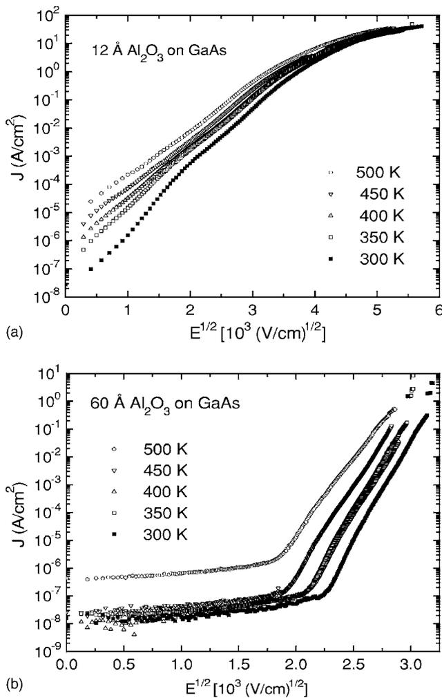
FIG. 1. (a) Measured leakage current density  $J$  vs square root of electric field  $E$  for 12 Å thick ALD Al<sub>2</sub>O<sub>3</sub> films on GaAs at five different temperatures (300 K  $\leq T \leq$  500 K). (b) The similar measurement performed at 60 Å thick ALD Al<sub>2</sub>O<sub>3</sub> films on GaAs.
