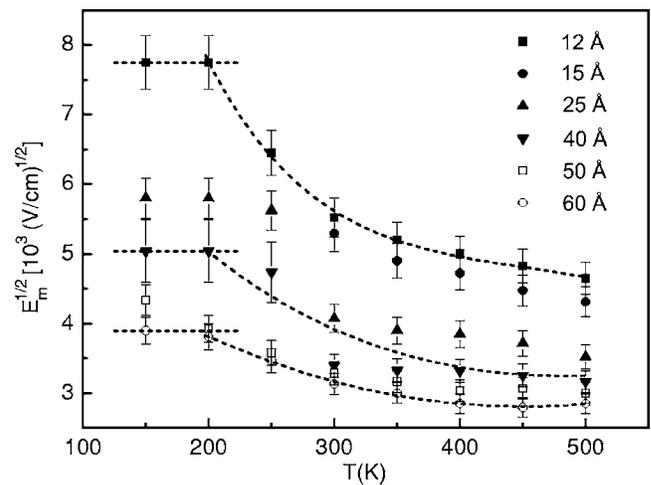
FIG. 2. Square root of the maximum dielectric strength  $E_m$  vs ambient temperature  $T$  for six different thickness ALD Al<sub>2</sub>O<sub>3</sub> films on GaAs. The dashed lines are calculated via Eqs. (1)–(3) on film thicknesses of 12, 40, and 60 Å using the experimental data except for  $C_1/\Gamma$  as a fitting parameter.
