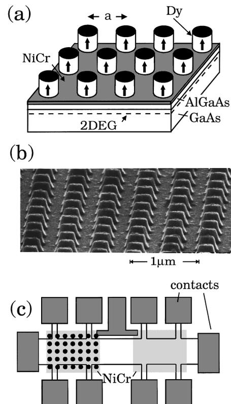
FIG. 1. (a) Sketch of the two-dimensional ferromagnetic Dy dot lattice on top of a GaAs–AlGaAs heterojunction. The corresponding electron micrograph of a tilted sample is shown in (b). Period of the square array: 500 nm; height of the dots: 200 nm. (c) Device geometry containing the Dy dot array and a NiCr coated, unpatterned reference area.
