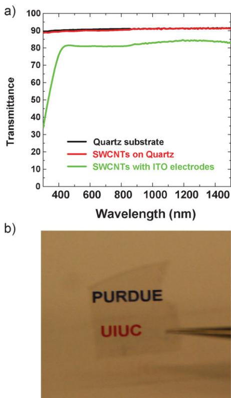
**Figure 4.** a) Optical transmission spectra as a function of wavelength through quartz substrates i) before and ii) after deposition of SWNT arrays and iii) after TFT fabrication. b) Photograph of a quartz substrate containing fully transparent SWNT-TFTs held over a sheet of paper containing printed text.
