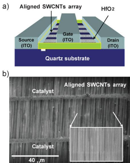
**Figure 1.** a) Schematic view of a top-gate TFT employing an aligned SWNT array with a  $\text{HfO}_2$  gate dielectric. b) SEM image of an aligned array of SWNT-TFT with an inset providing a higher magnification. The array contains  $\sim 0.5$  SWNTs  $\mu\text{m}^{-1}$ .
