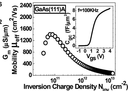
Fig. 7 Effective mobility  $\mu_{\text{eff}}$  from  $20\mu\text{m}$  gate length NMOSFET on GaAs(111)A. The peak electron effective mobility is  $1402 \text{ cm}^2/\text{Vs}$ .
