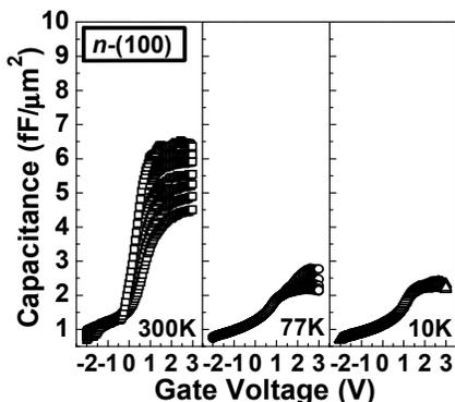
Fig. 9 C-V of Ni/8nm- $\text{Al}_2\text{O}_3/\text{n-GaAs}(100)$  measured at 300K, 77K, 10K. The significant drop of the accumulation capacitance is caused by the partial Fermi-level pinning at a certain location in the band-gap.
