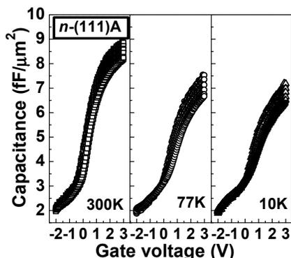
Fig. 8 C-V of Ni/8nm- $\text{Al}_2\text{O}_3/\text{n-GaAs}(111\text{A})$  measured at 300K, 77K, 10K. The small drop of the accumulation capacitance is caused by reduction of accumulation charge at low temperatures.
