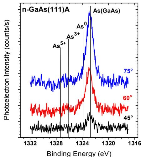
Fig. 17 As 2p XPS spectra at different take-off angles. Minimal As-oxides are detected at the interface for the GaAs(111)A surface. Similar results are seen for (110) and (100).
