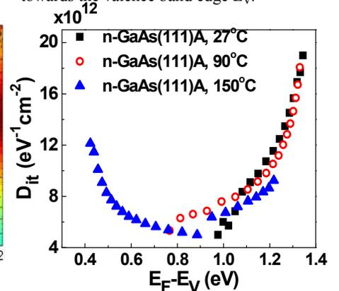
Fig. 15 Interface trap density extracted from temperature-dependent conductance method. There is no detectable peak distribution in the mid of band-gap. This is beneficial to move the Fermi-level on (111)A across the whole bandgap, compared to a possible peak distribution on GaAs(100) surface which is an obstacle to the Fermi-level movement.[7]
