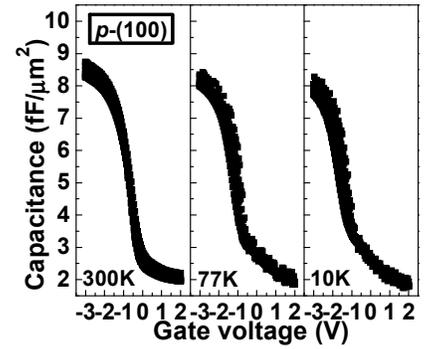
Fig. 12 C-V of Ni/8nm- $\text{Al}_2\text{O}_3$ /p-GaAs(100) measured at 300K, 77K, 10K. Unlike that on n-GaAs(100), there is only a small drop of the accumulation capacitance. This indicates that the Fermi-level is not pinned when moving towards the valence band edge  $E_V$ .
