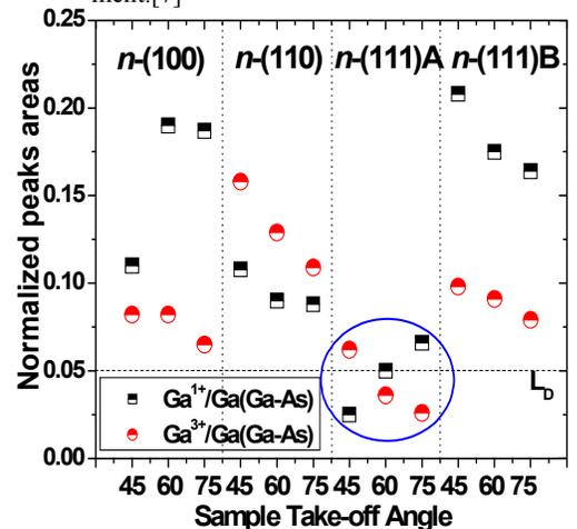
Fig. 18 Ga 2p XPS peak area ratios for various GaAs surface orientations and take-off angles. The GaAs(111)A surface has minimal Ga-oxide formation compared to the other orientations.  $L_D$  notes the detection limit. This correlates with the Fermi-level unpinning on GaAs (111)A from surface analysis.
