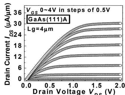
Fig. 4 Output characteristic ( $I_{DS} \sim V_{DS}$ ) for  $\text{Al}_2\text{O}_3/\text{GaAs}(111\text{A})$  NMOSFET with  $4\mu\text{m}$  gate length. The maximum drain current is  $30 \mu\text{A}/\mu\text{m}$ .
