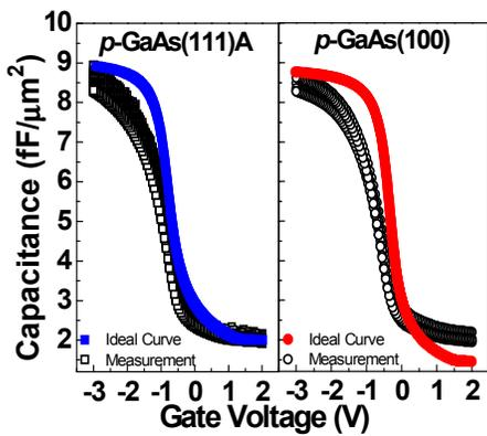
Fig. 13 Ideal high-frequency C-V plots at 27°C. On p-GaAs(111)A, the ideal curve fits very well at both accumulation and inversion sides, demonstrating that Fermi-level can move across the whole band gap. On p-GaAs(100), there is a discrepancy at inversion side, indicating the Fermi-level cannot reach strong inversion.
