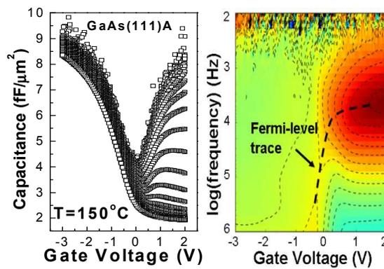
Fig. 14 C-V plot of Ni/8nm- $\text{Al}_2\text{O}_3$ /p-GaAs(111)A at 150°C (left). It shows clear inversion characteristics. The corresponding  $G-V$  plot from 100Hz to 1MHz (right) shows the Fermi-level trace turns to be independent of frequency at 10 KHz, demonstrating real minority carrier (electron) response from inversion.
