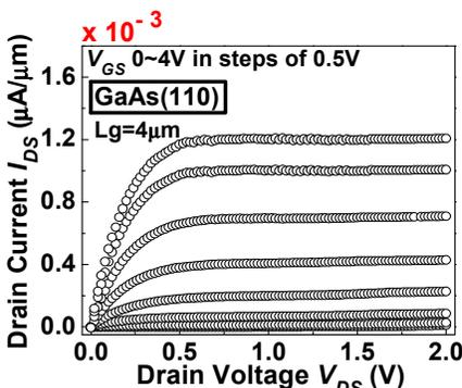
Fig. 3 Output characteristic ( $I_{DS} \sim V_{DS}$ ) for  $\text{Al}_2\text{O}_3/\text{GaAs}(110)$  NMOSFET with  $4\mu\text{m}$  gate length. The maximum drain current is  $1.2 \times 10^{-3} \mu\text{A}/\mu\text{m}$ .
