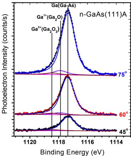
Fig. 16 XPS spectra of Ga 2p region at different take-off angles. Ga-oxides are near the detection limit for GaAs(111)A surface. More Ga-oxides are detected on (111)B, (110) and (100) surfaces.
