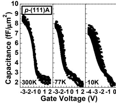
Fig. 11 C-V of Ni/8nm- $\text{Al}_2\text{O}_3$ /p-GaAs(111)A measured at 300K, 77K, 10K. Similar to that on n-GaAs(111)A, there is a small drop of the accumulation capacitance, which is caused by the reduction of accumulation charges at low temperatures.
