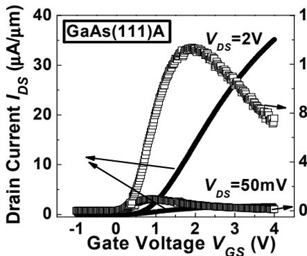
Fig. 6 Trans-conductance ( $G_m$ ) versus gate bias ( $V_{GS}$ ) of  $4\mu\text{m}$  gate length NMOSFET on GaAs(111)A. The peak  $G_m$  is  $14\mu\text{S}/\mu\text{m}$ .
