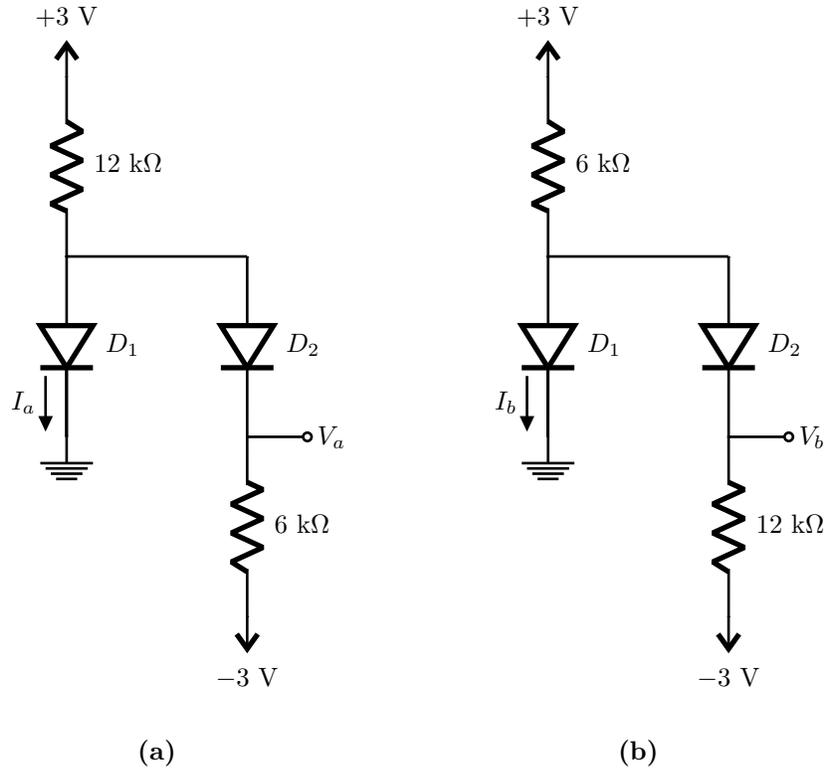
**Fig.1** - Simple Diode Circuits.
