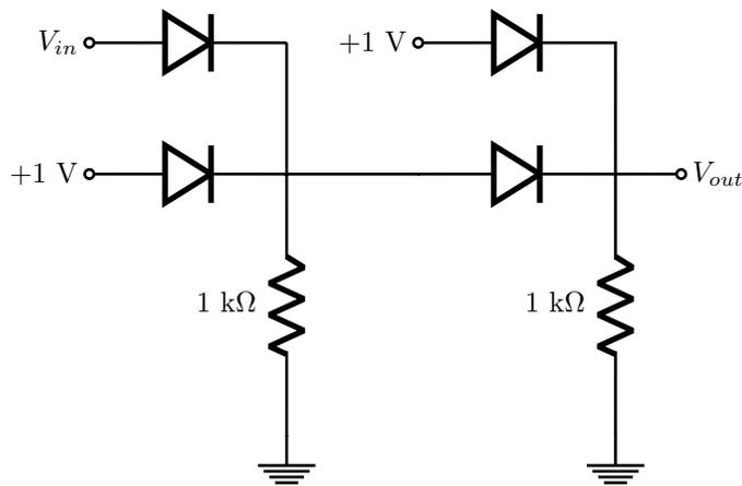
**Fig.9** - Cascaded OR Diode Gates.
