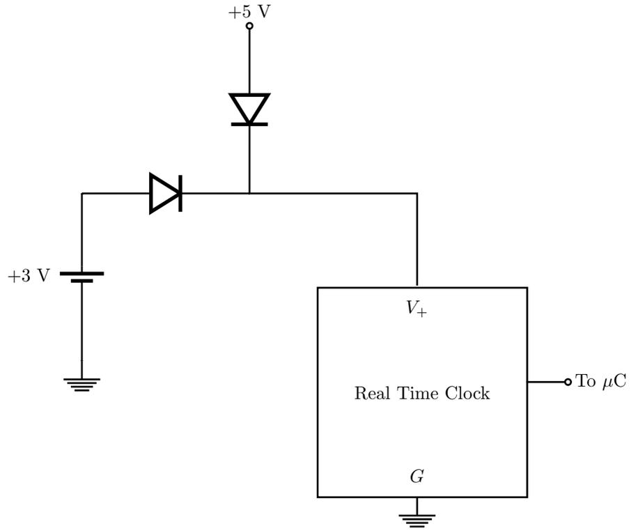
**Fig.10** - Battery Backup Circuit.
