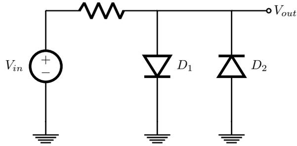
**Fig.4** - A simple voltage limiter.
