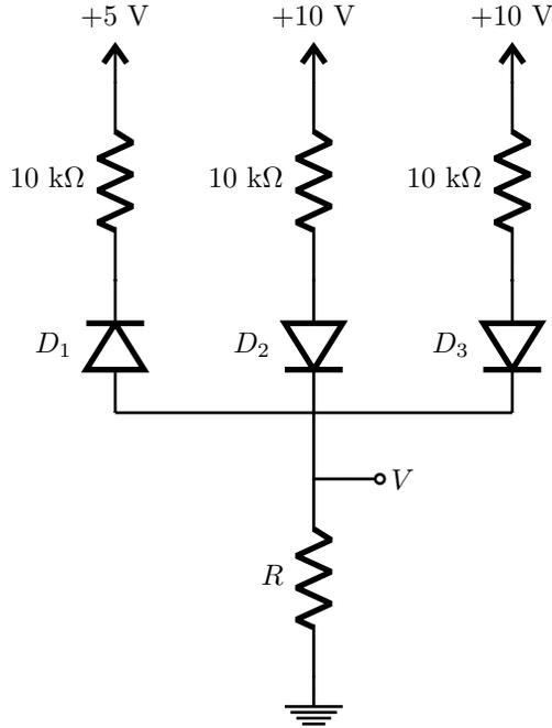
**Fig.2** - A More Complex Diode Circuit.
