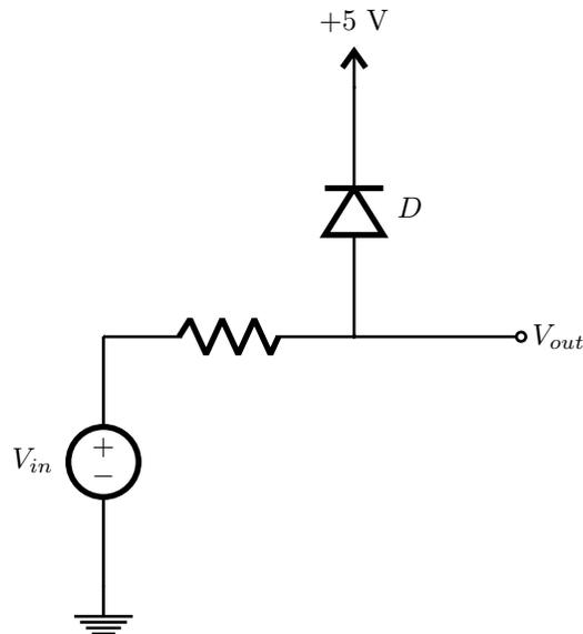
**Fig.5** - A simple voltage clamp.
