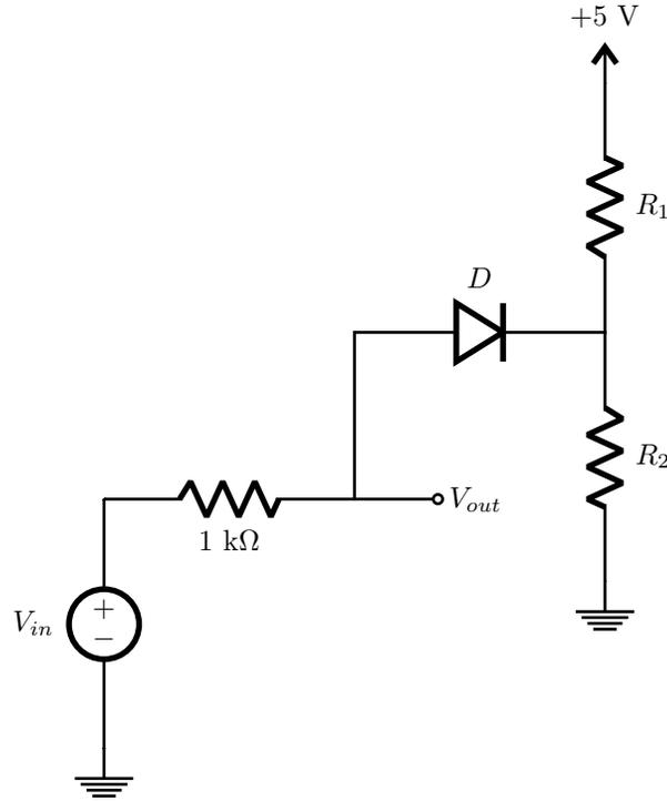
**Fig.6** - A simple voltage clamp with modified reference voltage.
