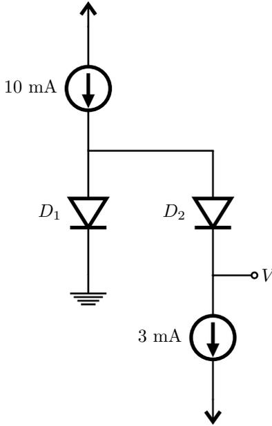
**Fig.3** - Circuit for which  $V_D = 0.7$  V Cannot be Assumed.
