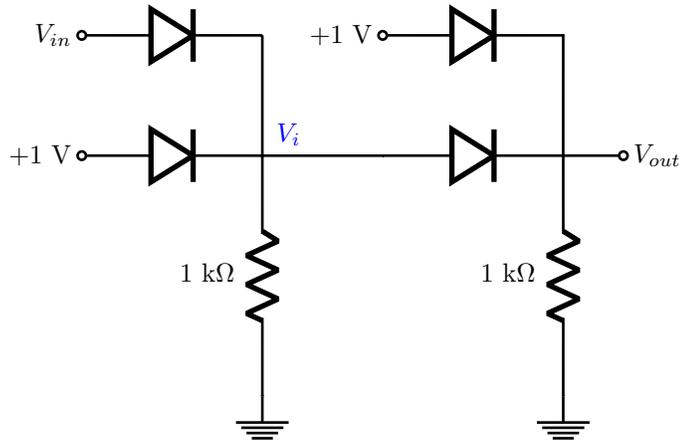
Fig.9 - Cascaded OR Diode Gates.
