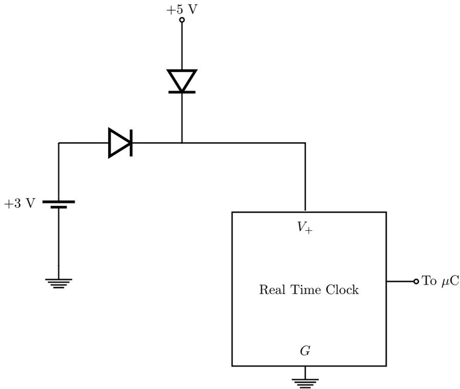
**Fig.10** - Battery Backup Circuit.
