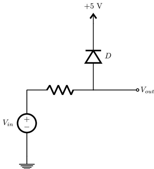
**Fig.5** - A simple voltage clamp.
