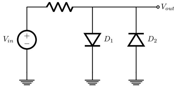
**Fig.4** - A simple voltage limiter.
