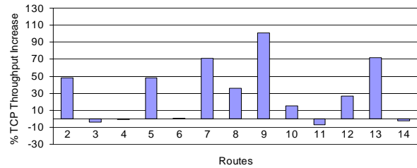
Figure 18: Testbed macrobenchmark: Basic scenario. TCP throughput gain on paths from node 1 to all other nodes.
