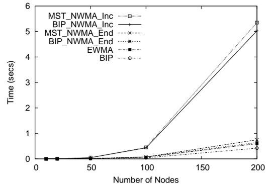
Fig. 3. Execution time of the six heuristics running on a 2Ghz Intel Pentium 4 PC.
