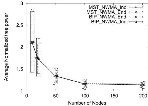
Fig. 2. Normalized tree power for 50 network instances and 10 and 90 percentiles.
