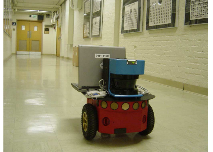
Fig. 13. Experimental environment and the Pioneer 3-DX robot with a SICK LMS-200 laser ranger. The boxes were placed to create corner features for prediction.
