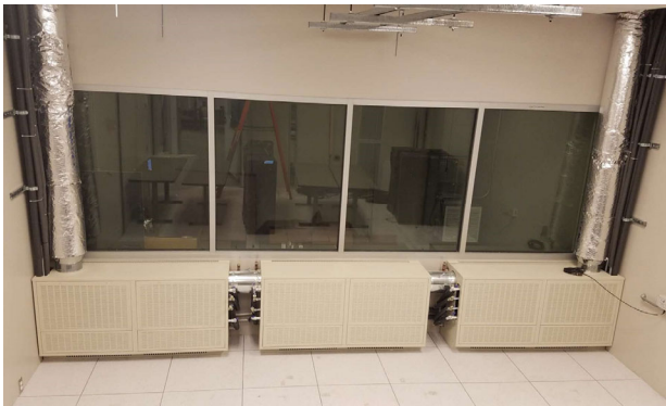
(a) DIV system inside IAQ chamber
