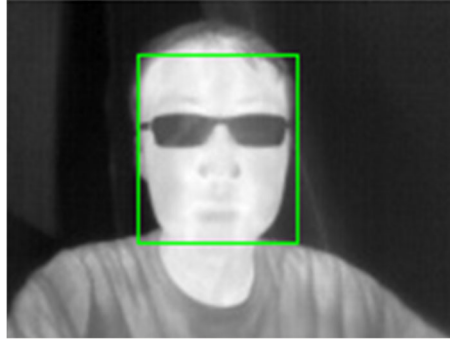
Figure 8. Detection of a face area for determining facial skin temperature.
