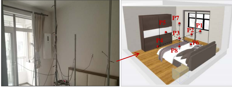
163 164 Fig. 2. Placement of indoor air temperature sensors 165
