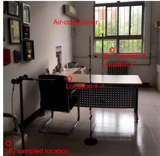
Figure 6. Inside view of the office and SF 6 sampling locations, with the SF 6 source released at the position from which this photo was taken.
