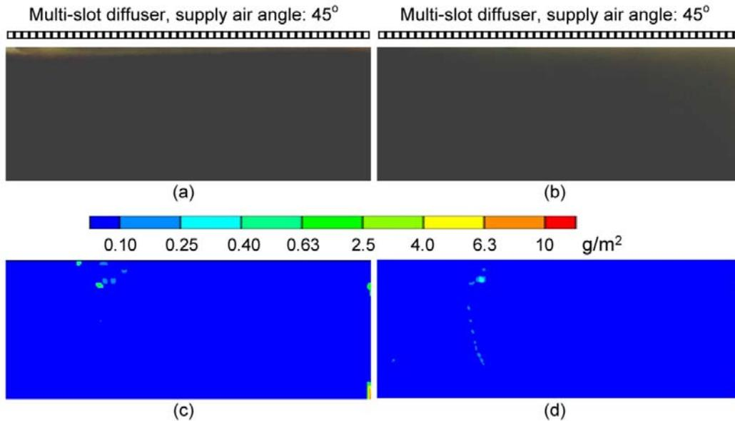
Figure 8. Comparison of experimentally determined and predicted particle deposition patterns on the left-hand wall under a slot diffuser supplying air at an angle of 45° for (a) PM<sub>2.5</sub> and (b) PM<sub>10</sub>.
