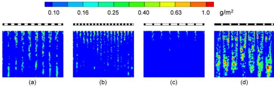
Figure 9. Distribution of PM<sub>2.5</sub> accumulation on the left-hand wall over a period of a month under different slot settings: (a) Case 1, (b) Case 2, (c) Case 3, and (d) Case 4.
