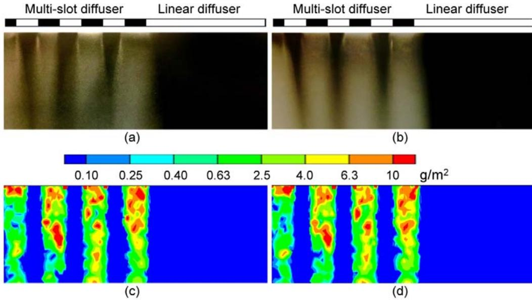
Figure 7. Particle deposition patterns on the left-hand wall under the multi-slot diffuser and the linear diffuser: (a) experiment for PM<sub>2.5</sub>, (b) experiment for PM<sub>10</sub>, (c) calculation for PM<sub>2.5</sub>, and (d) calculation for PM<sub>10</sub>.
