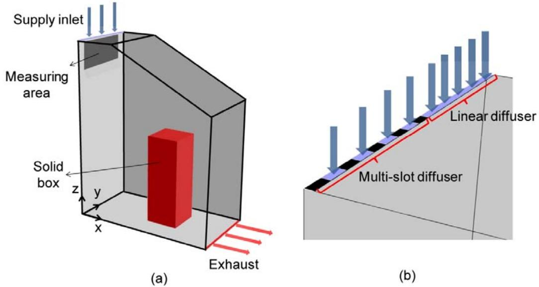
Figure 5. (a) The chamber configuration and (b) the air supply by means of a multi-slot diffuser (left) and a linear diffuser (right).
