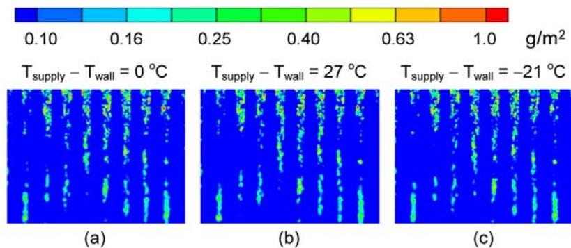
Figure 11. Distribution of PM<sub>2.5</sub> accumulation on the left-hand wall under the multi-slot diffuser over a period of a month under different temperature differentials between the supply air and the wall: (a) Case 1, (b) Case 8, and (c) Case 9.
