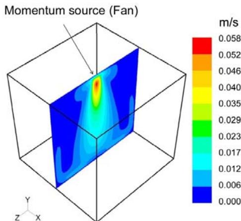
Figure 3. Configuration and airflow pattern of the chamber studied by You et al. [56].
