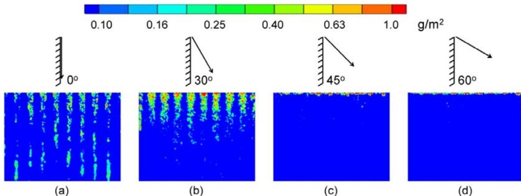
Figure 10. Distribution of PM<sub>2.5</sub> accumulation on the left-hand wall over a period of a month under different supply air angles: (a) Case 1, (b) Case 5, (c) Case 6, and (d) Case 7.
