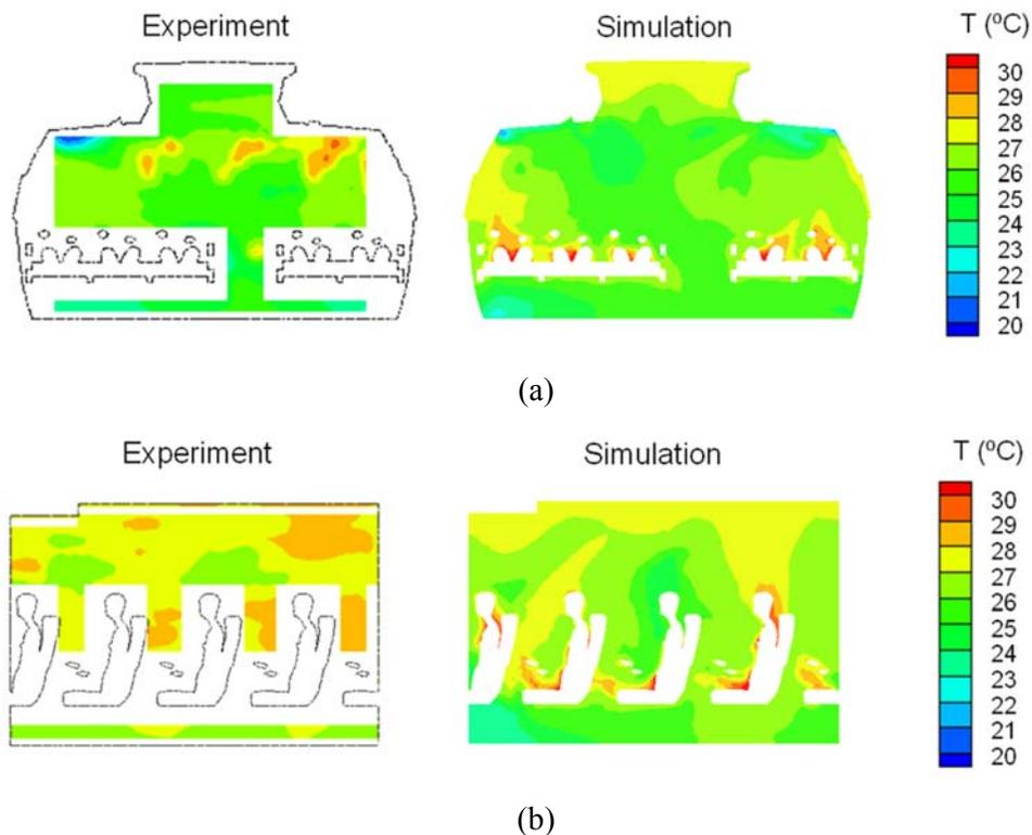
Figure 9 Comparison between the predicted and measured temperature field in (a) CS9, and (b) ASLS.
