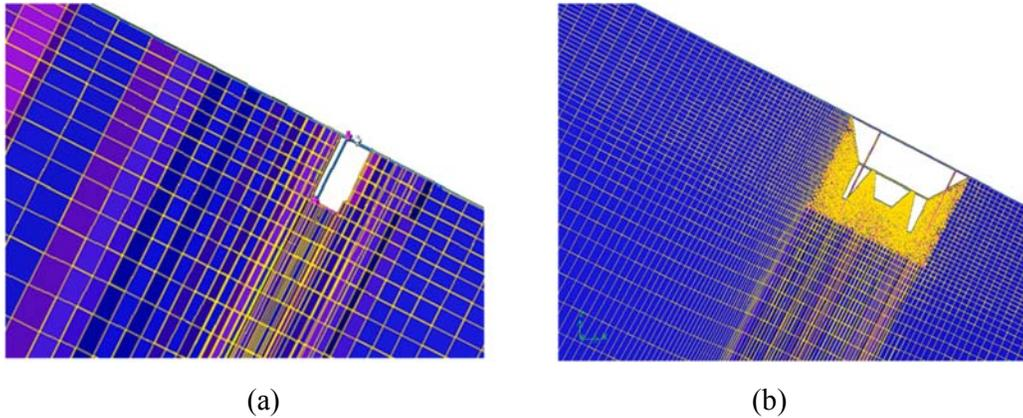
Figure 4 Comparison of the grid structure near the gasper for (a) the simplified gasper geometry model, and (b) the detailed gasper geometry model.
