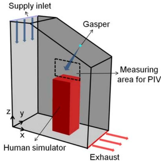
Figure 3 The sketch of the aircraft cabin mockup.
