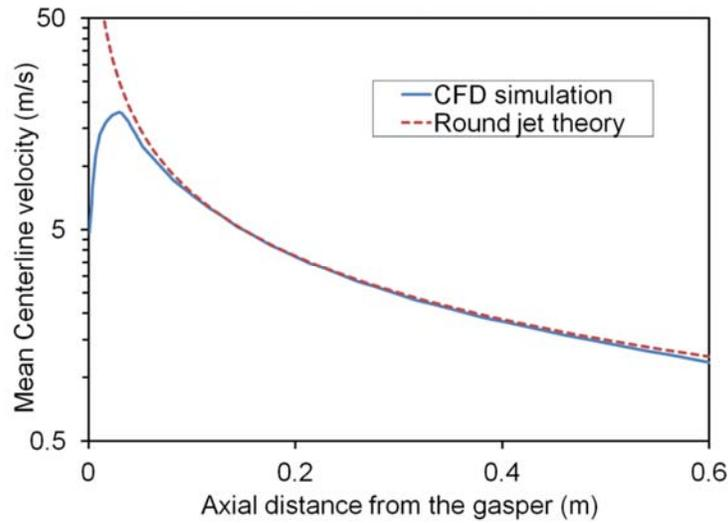
Figure 2 Centerline velocity decay as a function of axial distance for two types of jet.
