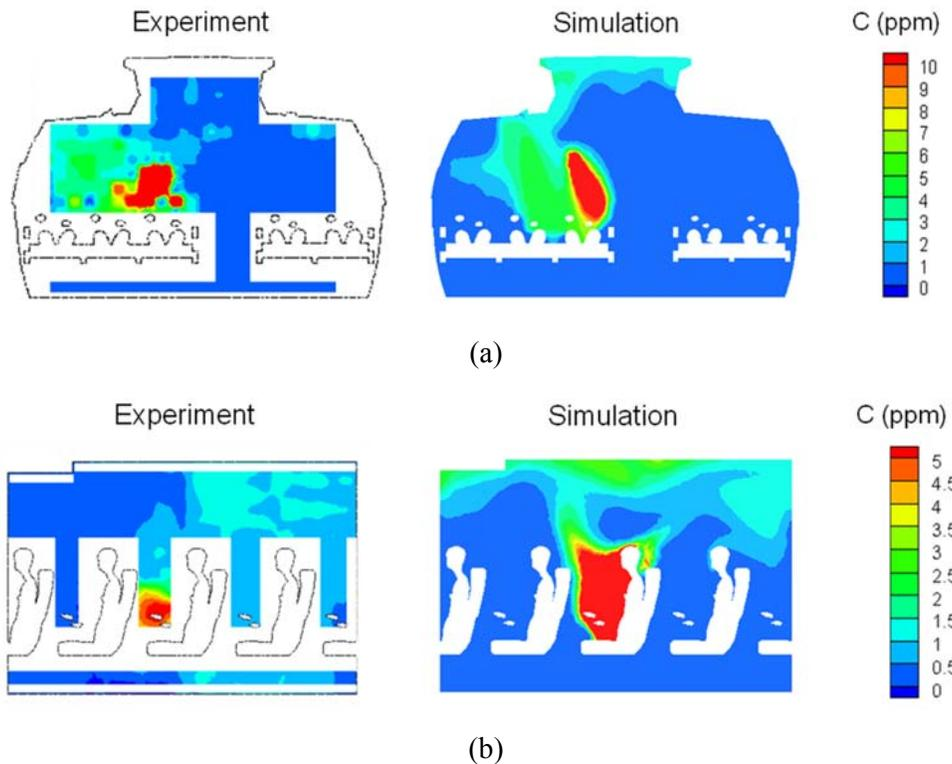
Figure 10 Comparison between predicted and measured contaminant concentration in (a) CS9, and (b) ASLS.
