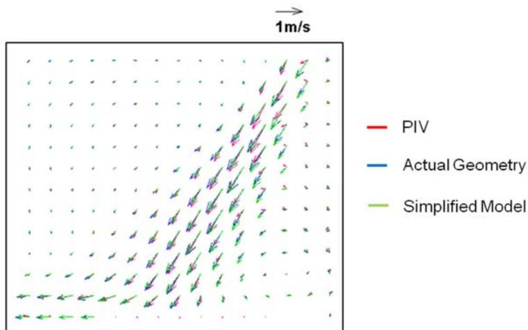
Figure 5 Comparison of the predicted airflow field by CFD with different gasper geometry models and experimental data in the critical area.
