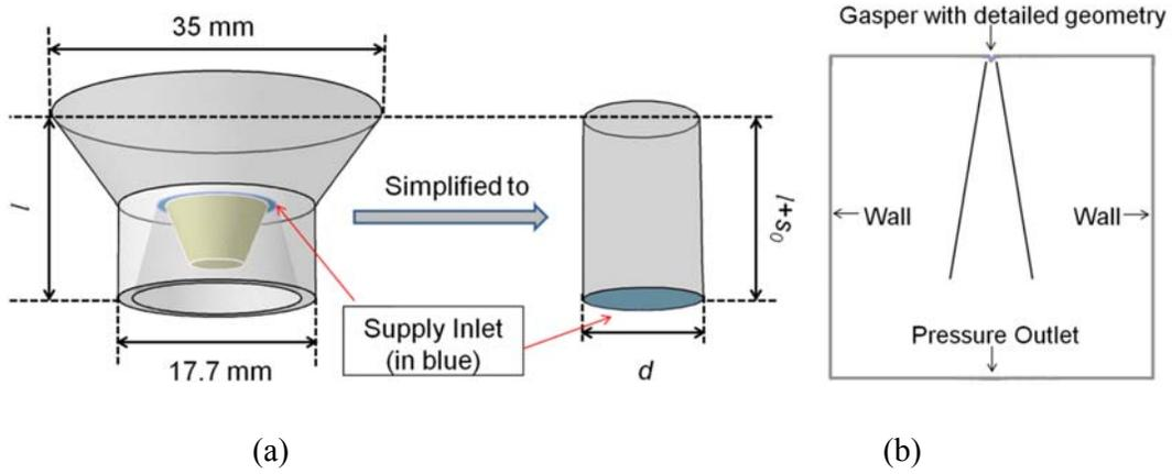
Figure 1 (a) Comparison of the detailed gasper geometry and the simplified gasper geometry; (b) case setup for studying the jet.
