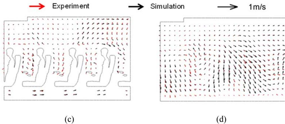
Figure 8 Comparison between the predicted and measured airflow field in (a) CS8, (b) CS9, (c) ASLS, and (d) CALS.
