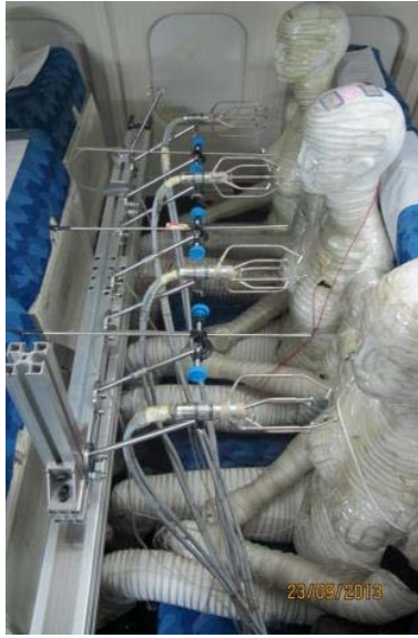
Figure 7 Setup of the sensor probes on the 3D robot system for measurements at a cross-section
