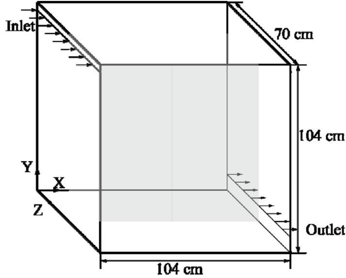
Figure 7. Schematic of mixed convection in a chamber with a heated floor
