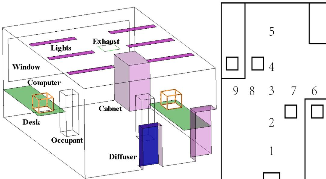
Figure 9. Schematic of displacement ventilation in the office space and measurement locations
