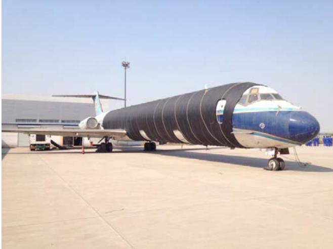
87 88 Fig.1 The insulated MD-82 aircraft facility with envelope 89
