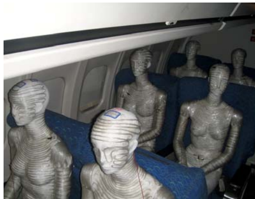
Figure 3. The first-class cabin with thermal manikins in a functional airplane at Tianjin University 9
