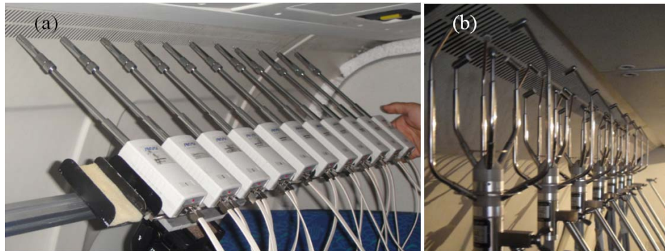
Figure 9 Instrument setup: (a) HSAs and (b) UAs
