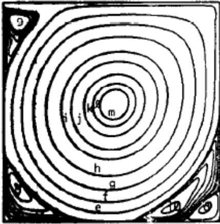
Fig. 10b Ghia's data [21] for streamlines for lid-driven cavity flow at Re = 10,000
