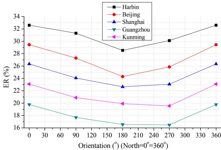
**Fig. 5** The energy performance of the dual-airflow window with different window orientations
