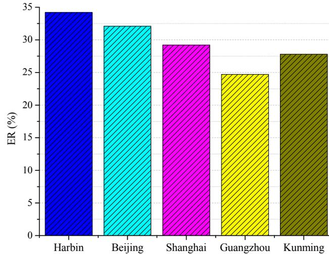
*Fig. 7 Energy saving with the dual airflow window compared with a conventional window under the optimal design parameters for different climate regions in China*
