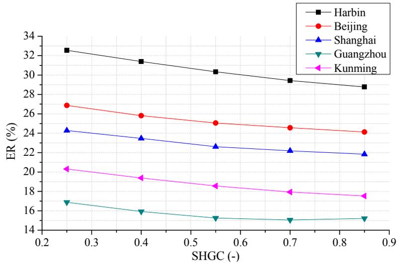
**Fig. 6** The energy performance of the dual-airflow window with different inner glass panes
