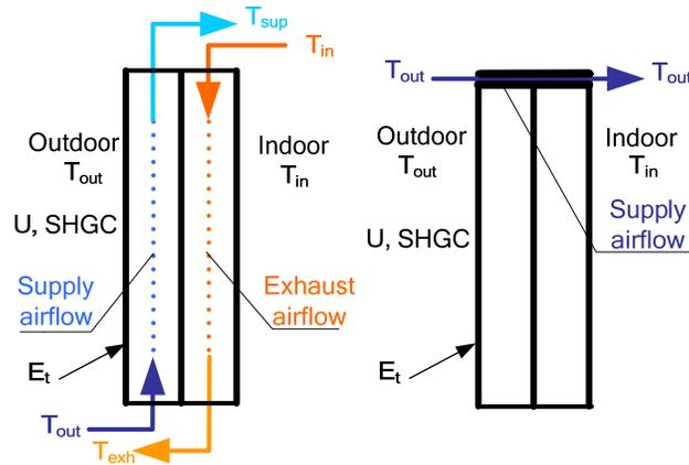
(a) Dual-airflow window (b) Three-layer conventional window
