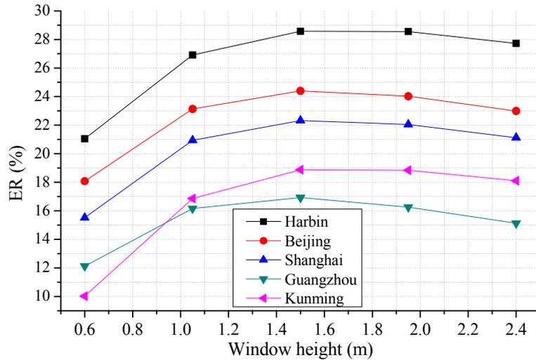
**Fig. 4** The energy performance of the dual-airflow window with different window heights
