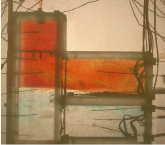
Fig. 2. Photograph of a small-scale model filled with water for flow visualization of a two-storey building with a common atrium (Livermore and Woods 2007)
