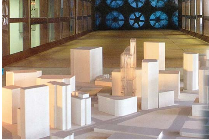
Figure 4. A building site model within a wind tunnel.
