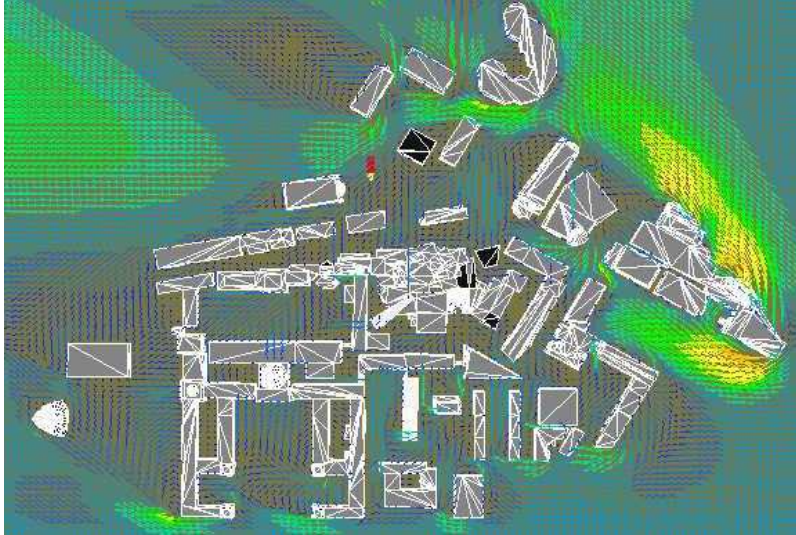
Figure 6. Wind distribution around Stata Center at the ground level (yellow – high wind speed, green – moderate wind speed, and blue – low wind speed).
