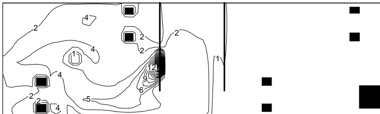
C3 concentration contour at occupant head section at t = 5 mins with EASE Strategy3
