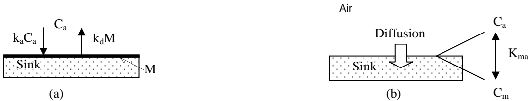
Figure 2. Schematic of the sorption process considered by (a) first order adsorption/desorption rate models, and (b) equilibrium-interface models.
