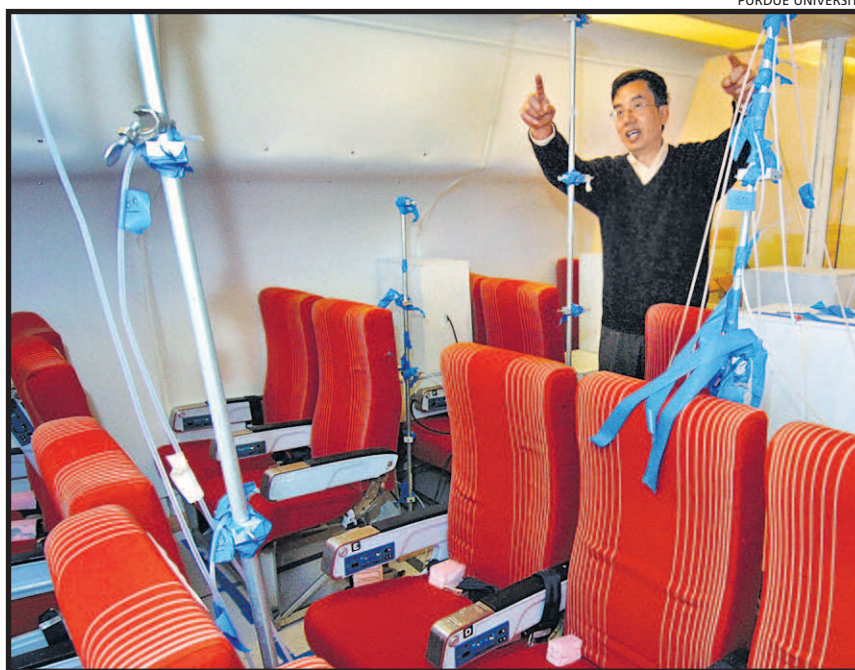
Qingyan Chen describes the workings of his Purdue lab, which recreates the passenger area of an airliner. The research aims to develop a system that locates passengers releasing hazardous materials or pathogens inside airline cabins. The technique might enable officials to identify passengers responsible for the unintentional release of germs or the intentional release of pathogens or chemical agents, such as those used in a terrorist attack
