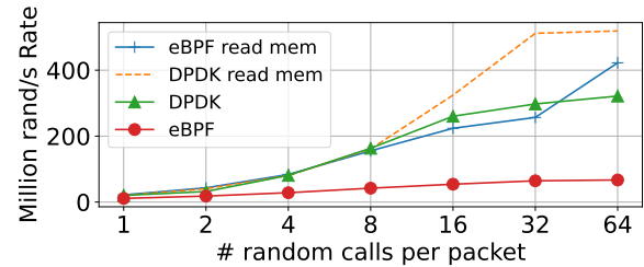
Figure 5: eBPF and DPDK performance when generating different number of random 32-bit numbers per packet using the same prandom_u32 function. The eBPF/DPDK read mem plot indicate the performance when reading pre-generated random bits from memory.
