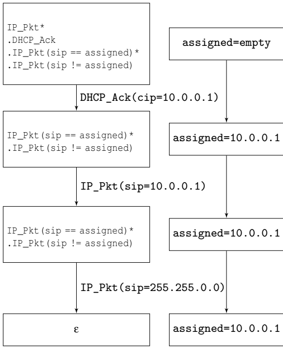
Figure 4: The progress of matching a string with the DHCP example. The left column contains the binding-free patterns, and the right tracks the environment. The arrows indicate the pattern derivative with the incoming event and current environment. Acceptance is indicated by the empty string, \epsilon .
