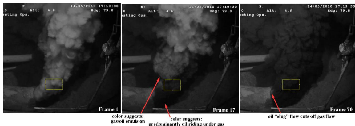
Fig. 1 - Plume of oil and gas escaping the riser pipe showing the three flow types, gassy, transition, and slightly oily. Also shown is the location of interrogation window.
