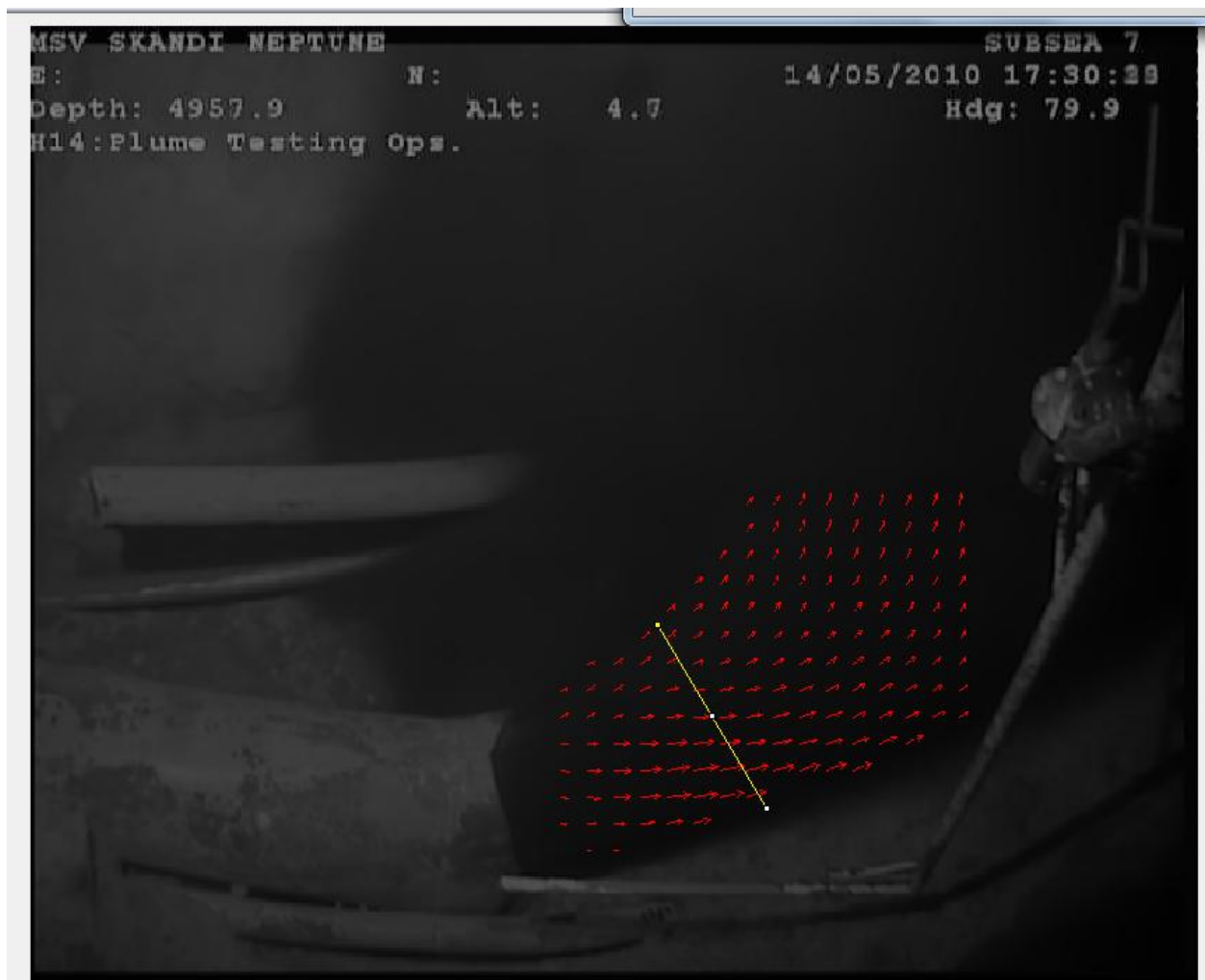
Fig 3. Displacement (or velocity) field and plume diameter measurement area. The average velocity is 7.52 in/sec and the plume diameter is 24.53 in along the yellow line.
