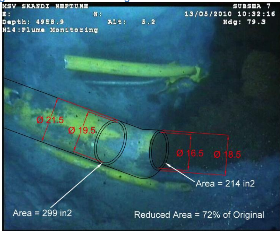
Figure 2: Riser outlet showing its reduced cross-sectional area
