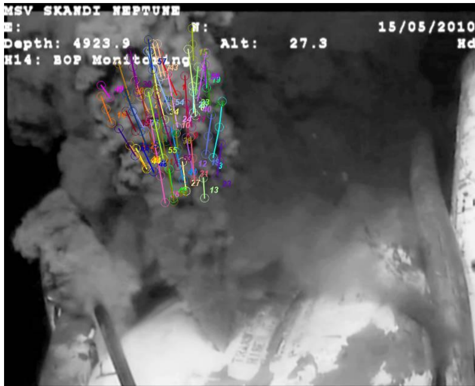
Figure 6: Feature tracks manually identified in the main jet of the Riser Kink Jet. (The trajectories of features shown in this image were pseudocolored randomly so they are easier to see. The colors do not represent velocity magnitude)
