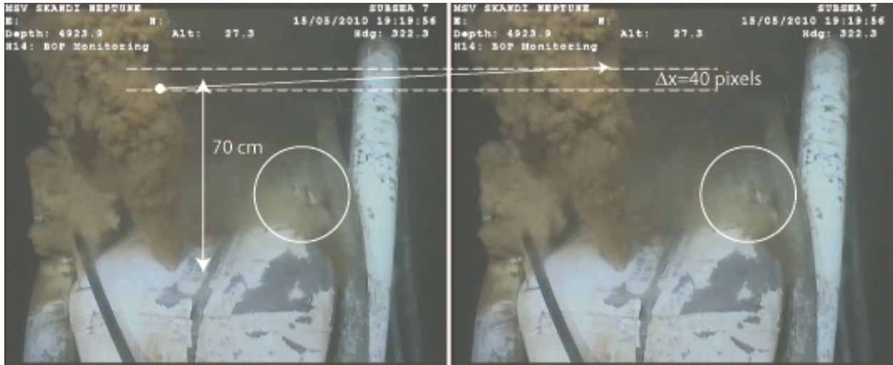
Figure 2: Two successive images from a video sequence (24 fps), showing the advection of large structures downstream of J_1 . Circles mark a group of dark patches that can be tracked individually.
