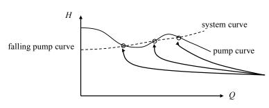
For the system shown at the left there are three operation points! The system may oscillate between these points!
